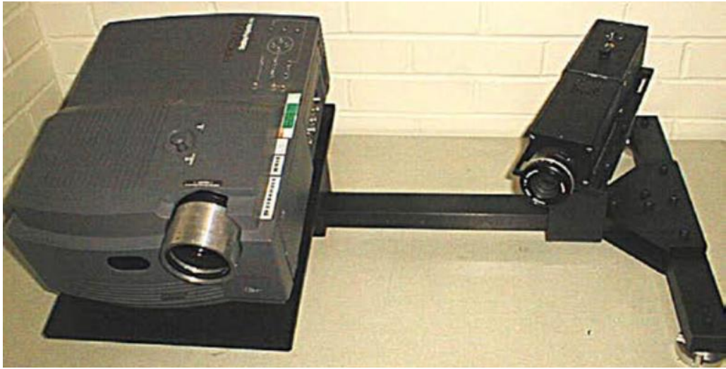
Figure 6-1: Initial prototype optical SMS developed by Coggrave in 2001 [10].
