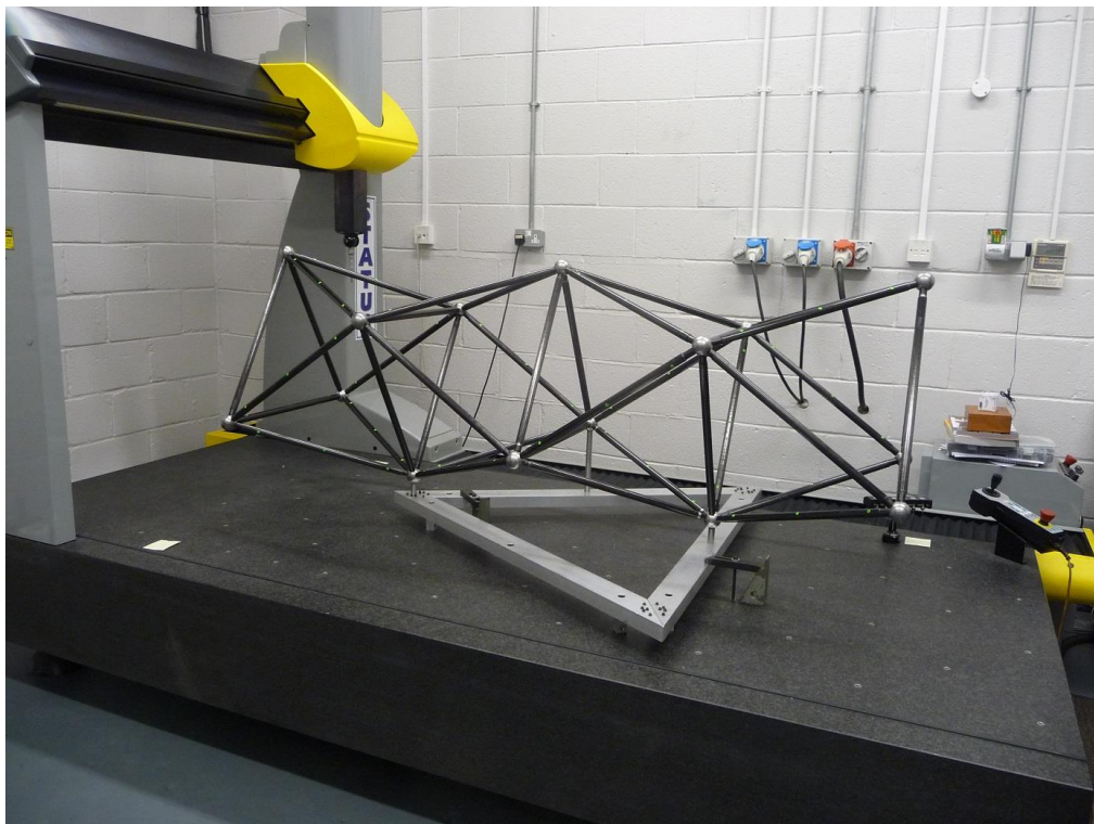
Figure 3-9: CMM characterisation of the large volume calibration artefact.
