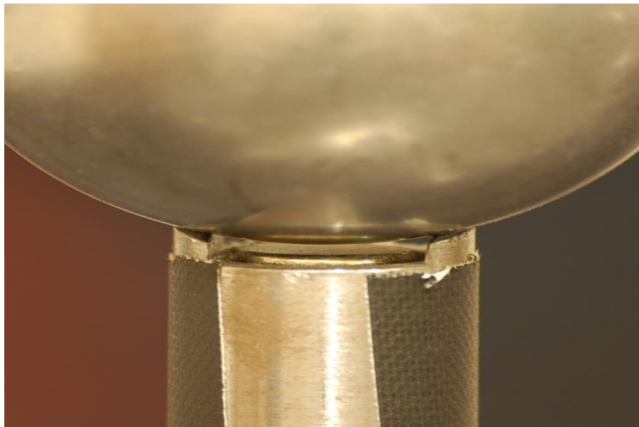
Figure 4-8: The second support, manufactured to provide two of the rigid body constraints in translation. (a) Support without sphere positioned showing the magnet which provides the contact force between the sphere and the two contact areas of the support. (b) Support with sphere positioned highlighting the contact between the two mating surfaces.
