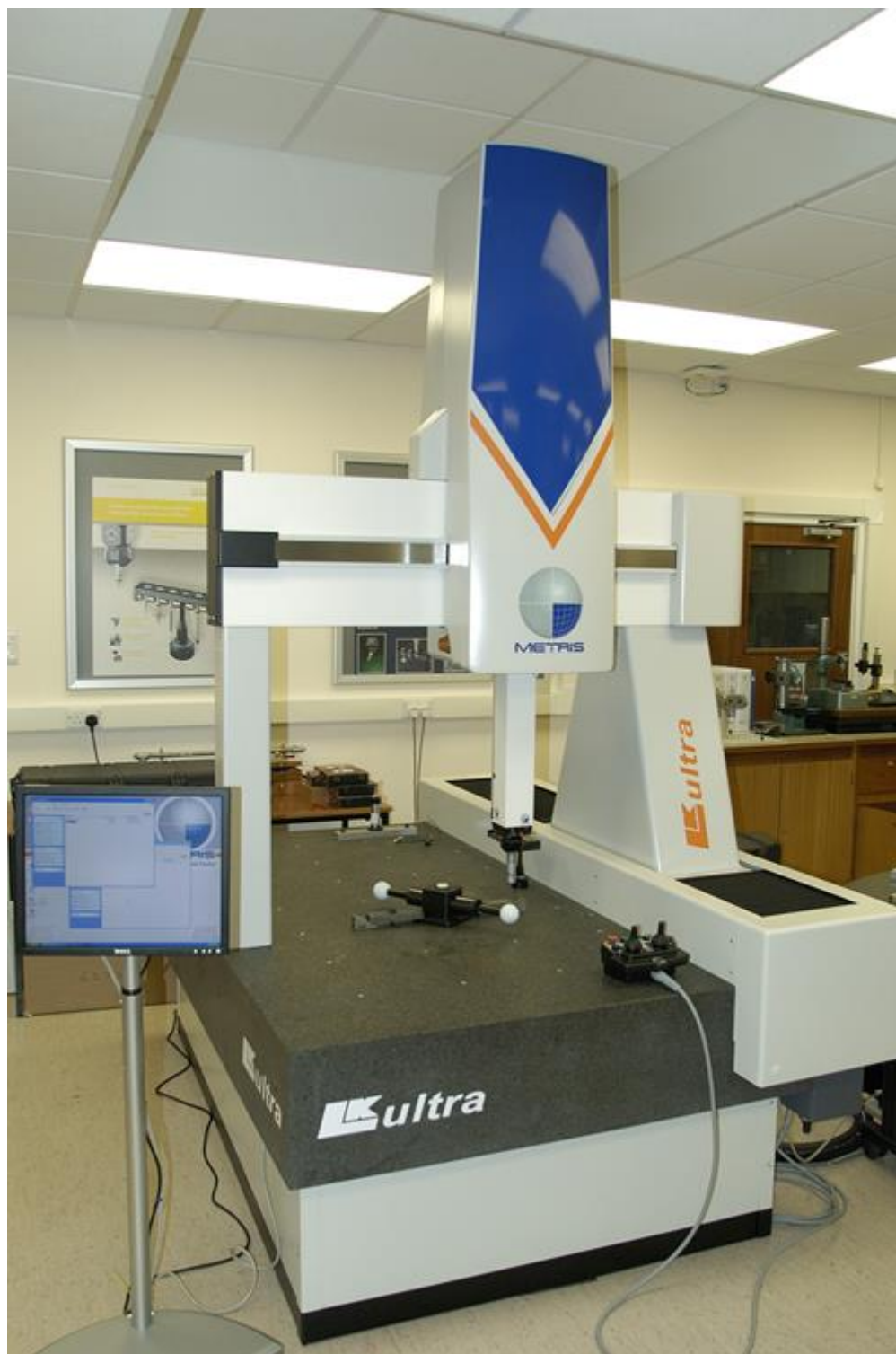
Figure 1-2: A mechanical CMM with a bridge structure.
