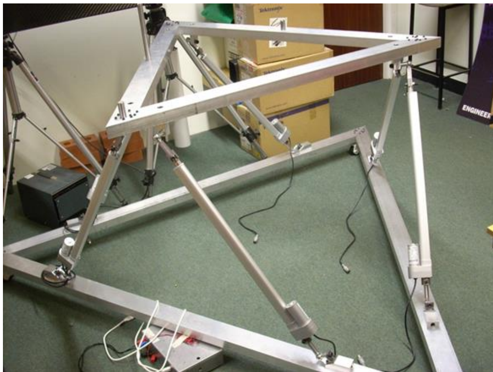
Figure 4-2: Fully functional Stewart platform manipulator with six DOF.
