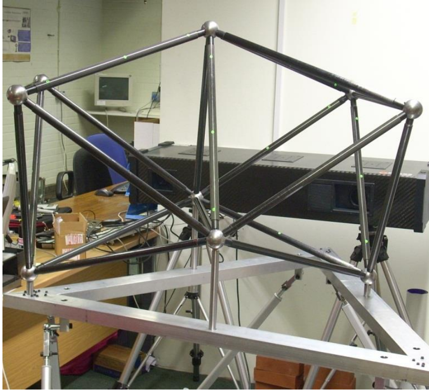
Figure 3-8: Double octahedral calibration artefact – supported by the manipulator.
