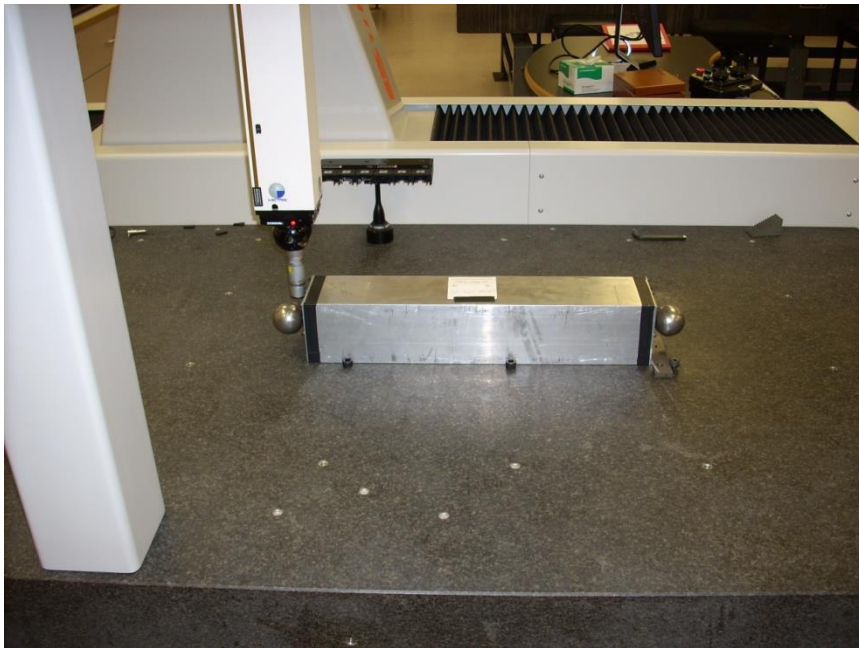
Figure 3-12: CMM measurements of the dimensional changes from thermal and hygral effects.
