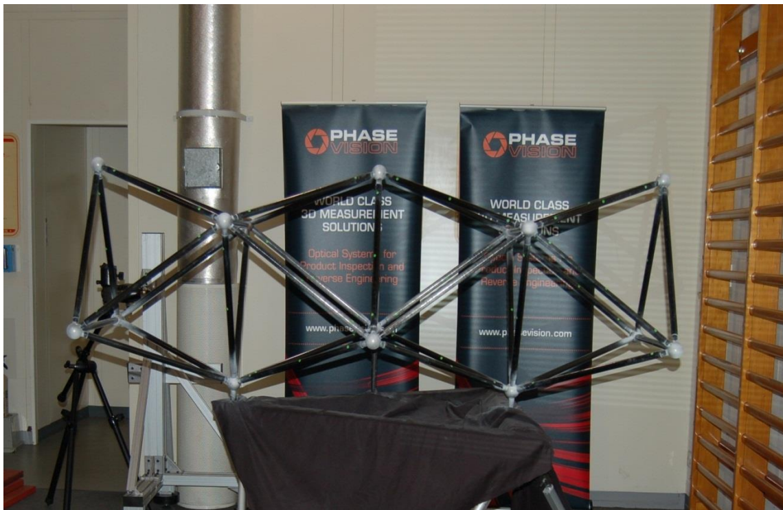
Figure 6-4: View of large volume calibration artefact from behind the optical SMSs.
