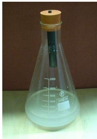
Figure 3-13: Humidity chamber used to test samples of carbon fibre at 25% and 75% RH.
