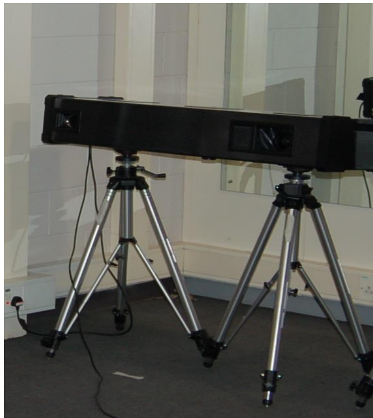
Figure 6-2: Latest SMS1200 DBE scanner, of which two were used in this work.
