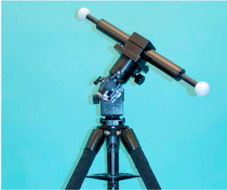
Figure 3-1: Phase Vision Ltd – Ball-bar calibration artefact.
