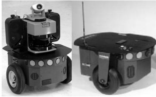
Fig.3 Pioneer 3-DXmobile robots [9] or cite where these pictures were took from as they not produced by you
