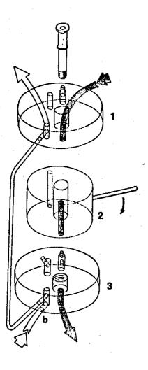
Figure 8.2 Double-injection valve
