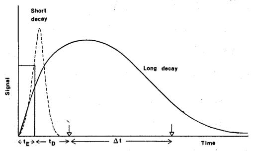
Fig 1.2 Diagram of time resolved fluorescence measurements  $t_E = Excitation pulse time (<1 ns)$   $t_D = Delay time$  $\Delta t = Counting time interval$
