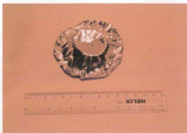
Figure 11.35 Rear view of the thin aluminium projectile after a 3kV launch
