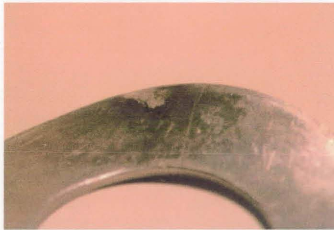
Figure 11.10 A close-up of the damage to the projectile caused by an arc.
