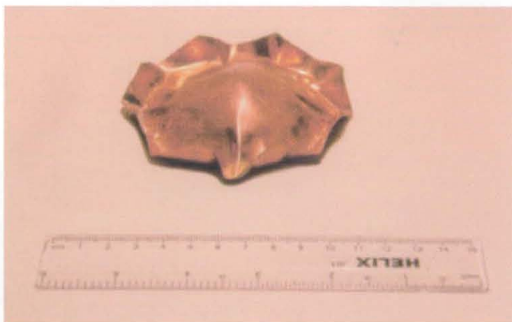
Figure 11.38 An octagonal projectile after launch
