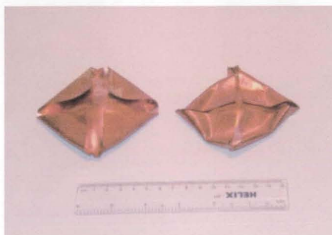
Figure 11.40 Square copper projectiles after launch
