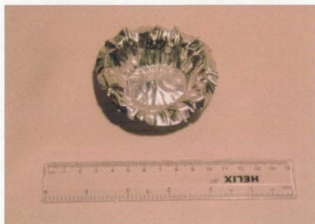
Figure 11.34 Front view of the thin aluminium projectile after a 3kV launch
