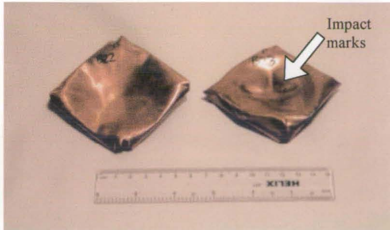
Figure 11.42 Front view of square copper projectiles after launch
