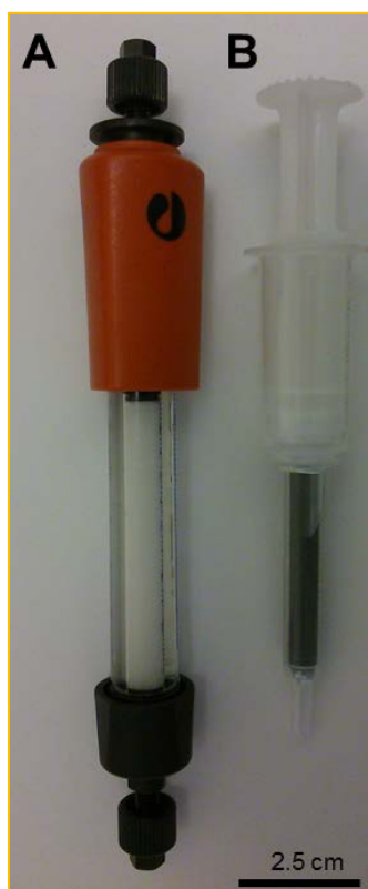
Figure 5.1: Comparison of chromatography and MACS ® column. (A) Tricorn 5/50 column with adjustable adapter on the top packed with modified and functionalized glass beads. (B) MACS ® LS column with the inserted plunger for the mechanical elution of cells of interest.
