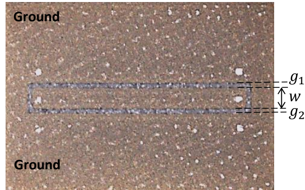
Figure 7.20 Optical microscope image of a printed CPW line (2 mm long)
