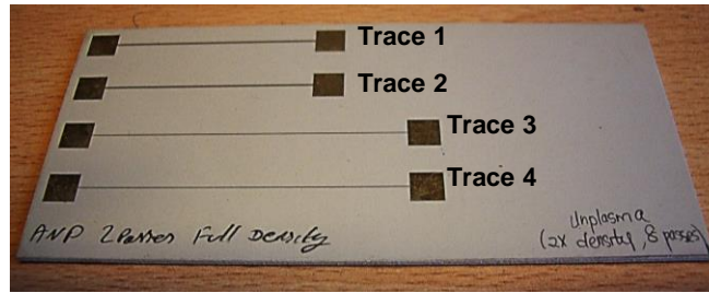
Figure 5.5 Printed two point probe test structures
