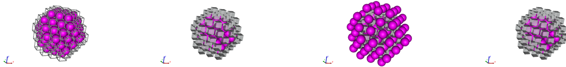
Figure 7.3: The configurations of bubble Xe_{116}V_{116} . From left to right: spherical way before minimisation, spherical way after minimisation, cuboctahedral way before minimisation, cuboctahedral way after minimisation. The grey cubes represent Al vacancies and pink spheres are Xe atoms.
