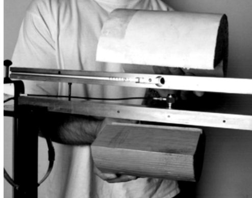
Figure 2.13 - Surrogate thigh components developed by Hrysomallis (2009) showing Silastic 3483 soft tissue surface, wooden surrogate backing, and steel skeletal component ( Image reproduced with permission of the rights holder, Elsevier ).
