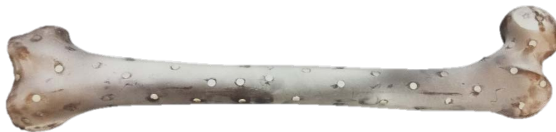
Figure 8.2 - Composite femur coated in developer spray and retroreflective markers.
