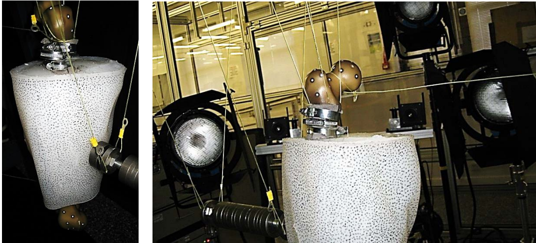
Figure 9.4 – Images showing the speckle pattern on surrogate surface for GOM ARAMIS DIC tracking and the camera and lighting orientation.
