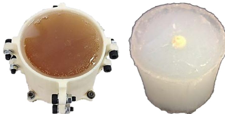
Figure 8.13 - Small scale cylindrical surrogate with 1.5mm skin layer.
