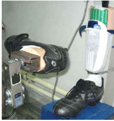
Figure 2.14 - Durable surrogate lower leg developed by Tatar et al. (2014) with boot mounted pendulum end-effector (Image reproduced with permission of the rights holder, JSSM).
