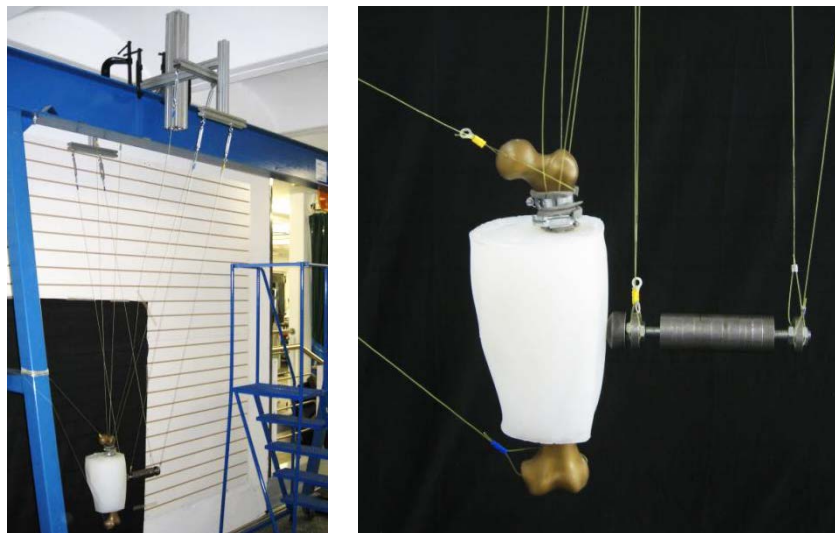
Figure 9.1 – Pendulum test rig configuration with mounted striker and surrogate bodies.
