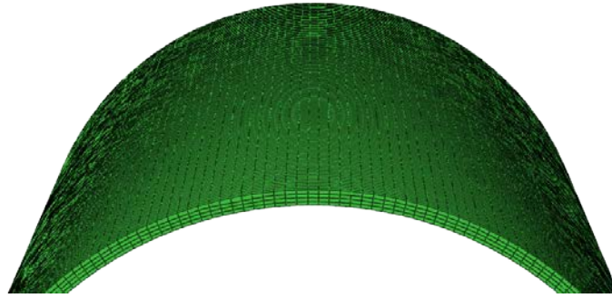
Figure 4.10 - Four continuum solid elements through skin layer.
