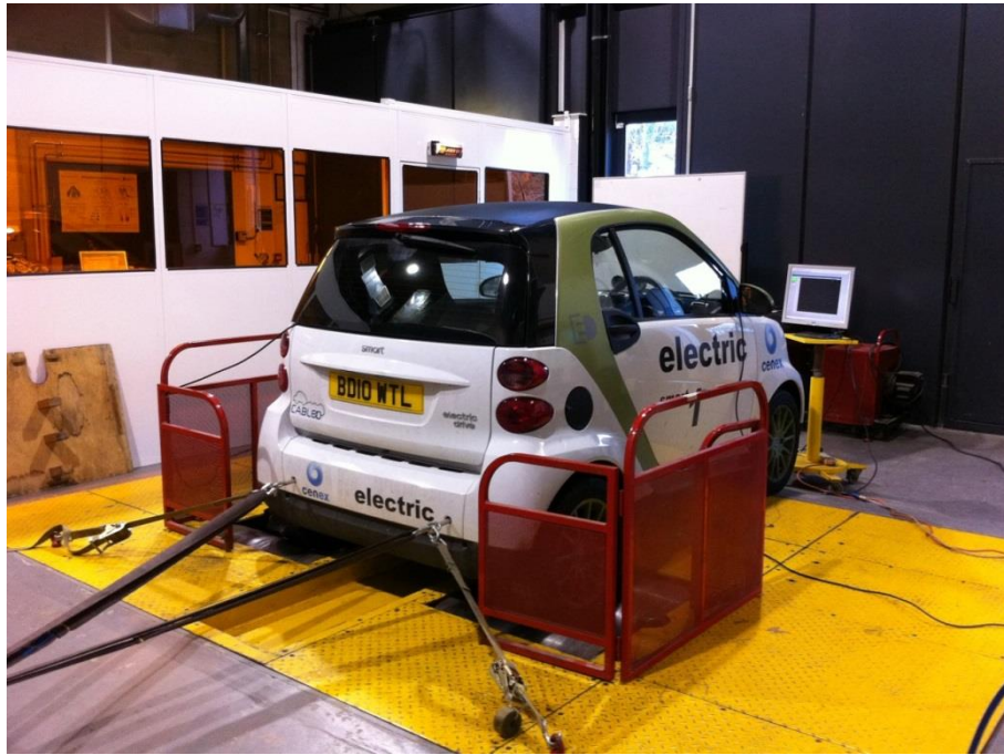
Figure 3.18: Smart electric drive on Loughborough University chassis dynamometer
