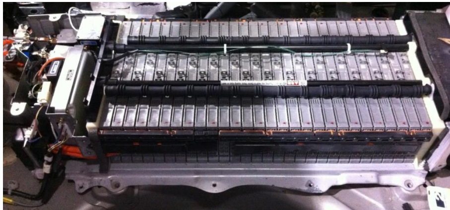
Figure 2.2: Prius HV battery pack in situ in the car with the cover removed
