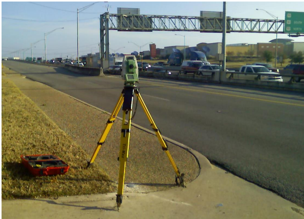
Figure 3.20: Surveying using total station [73]
