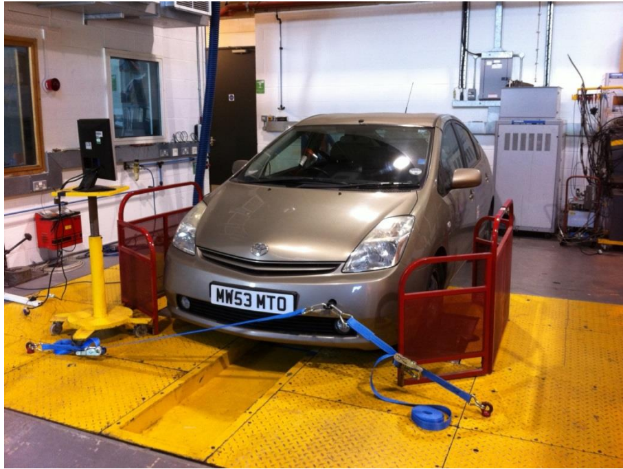
Figure 3.16: Toyota Prius II test car on Loughborough University chassis dynamometer
