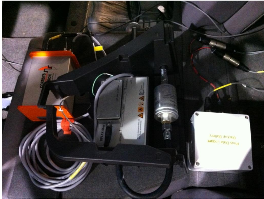
Figure 3.17: Fuel flow instrumentation set up for chassis dynamometer testing
