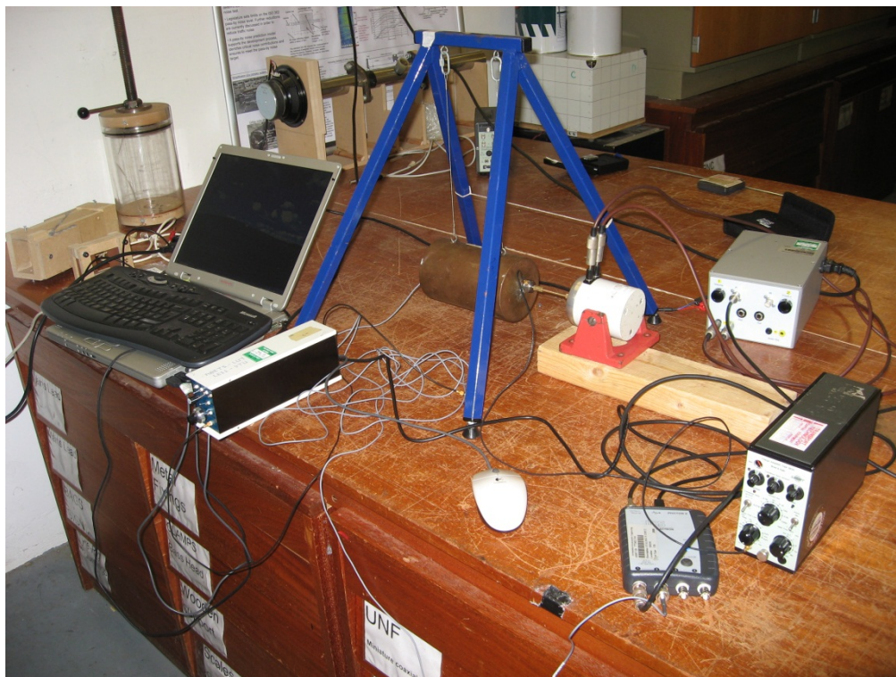
Figure 122: Apparatus for the calibration of force transducer
