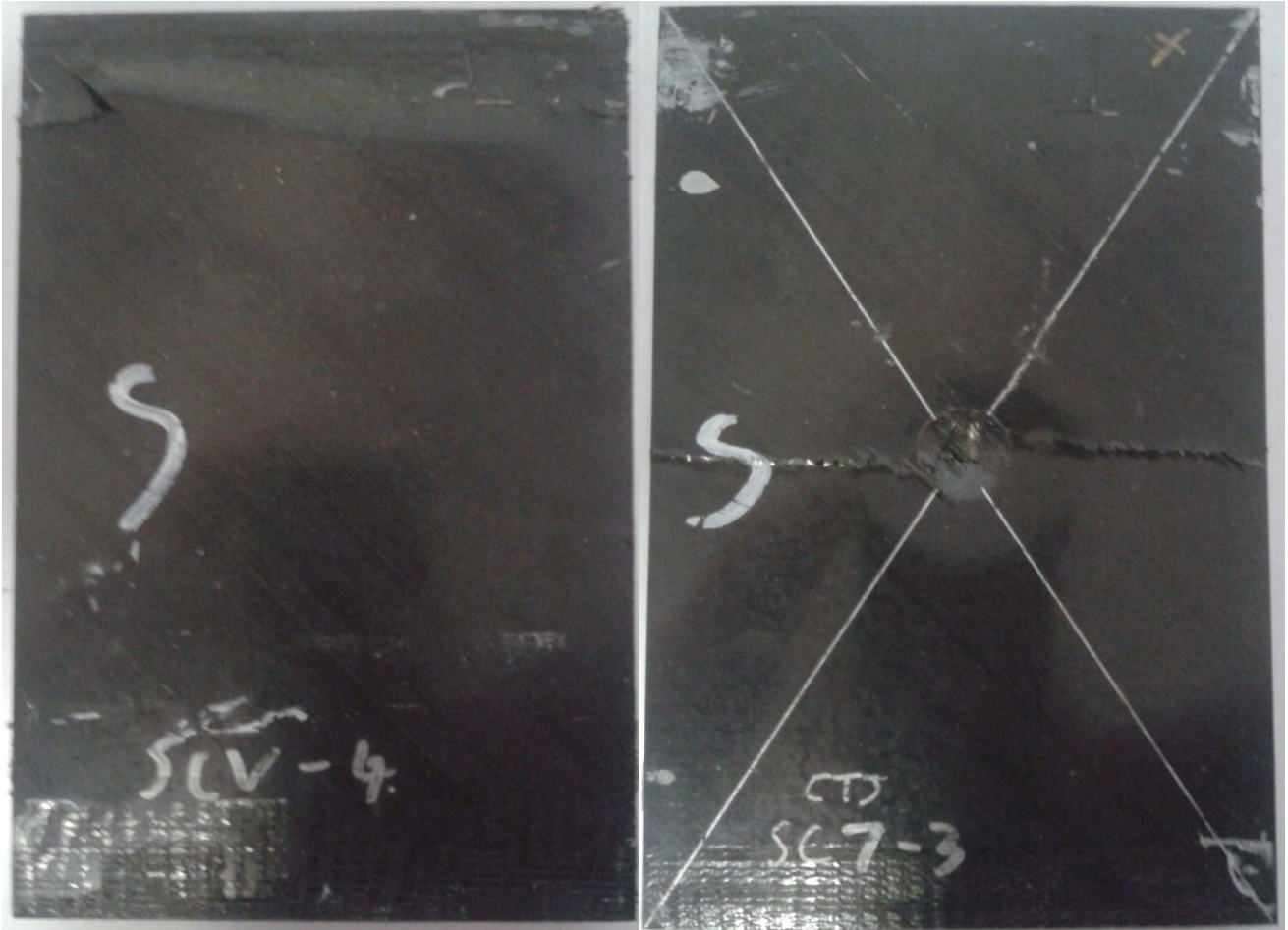
Figure 37: Failure of sandwich panels a) (left) delamination buckle towards the top end of the panel, b) (right) kink-band propagation originating from the damaged region [2]
