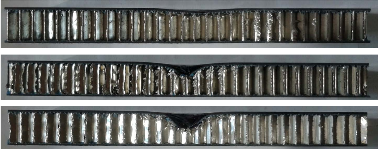
Figure 30: Sectioned asymmetric panels after impact (from top) a) 4J, b) 7J, c) 10J initial kinetic energy
