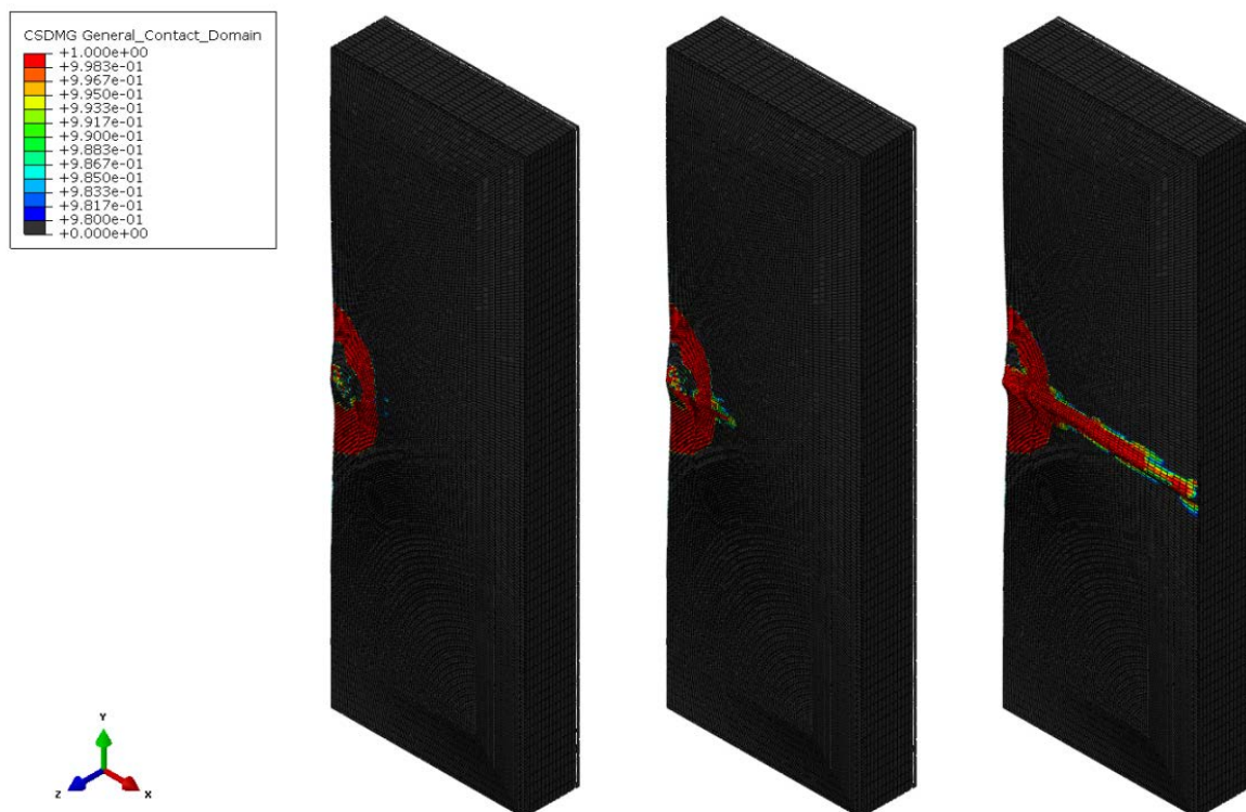
Figure 91: Delamination propagation in S7-C . The leftmost frame shows the panel just prior to final failure, with the delamination growing outwards from the damaged region to the fully-developed state in the rightmost frame. The failure propagated fully in less than 0.2ms. [2]
