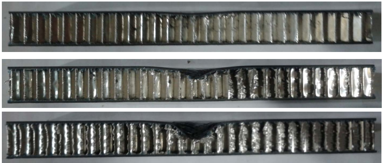
Figure 29: Sectioned symmetric panels after quasi-static-indentation (from top) a) 2.5mm, b) 5mm, c) 7mm applied displacement [2]
