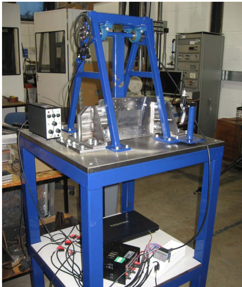
Figure 23: Pendulum impact jig
