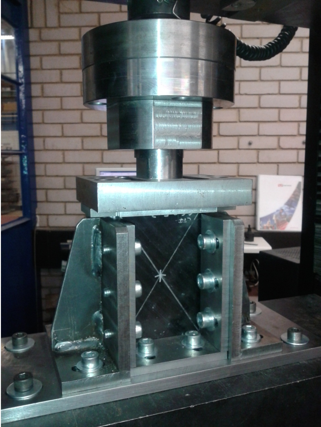
Figure 36: A panel loaded into the compression-after-impact support fixture, ready for testing [2]
