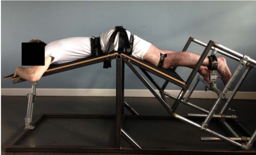
Figure 7.1. Isometric measurements of the knee flexors were made with this custom-made isometric dynamometer in the joint configuration shown. Isovelocity torque measurements were made with a Con-Trex isokinetic dynamometer.
