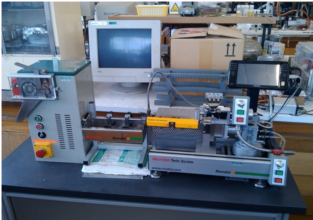
Fig.3.2:Lab scale twin screw extruder for melt blending
