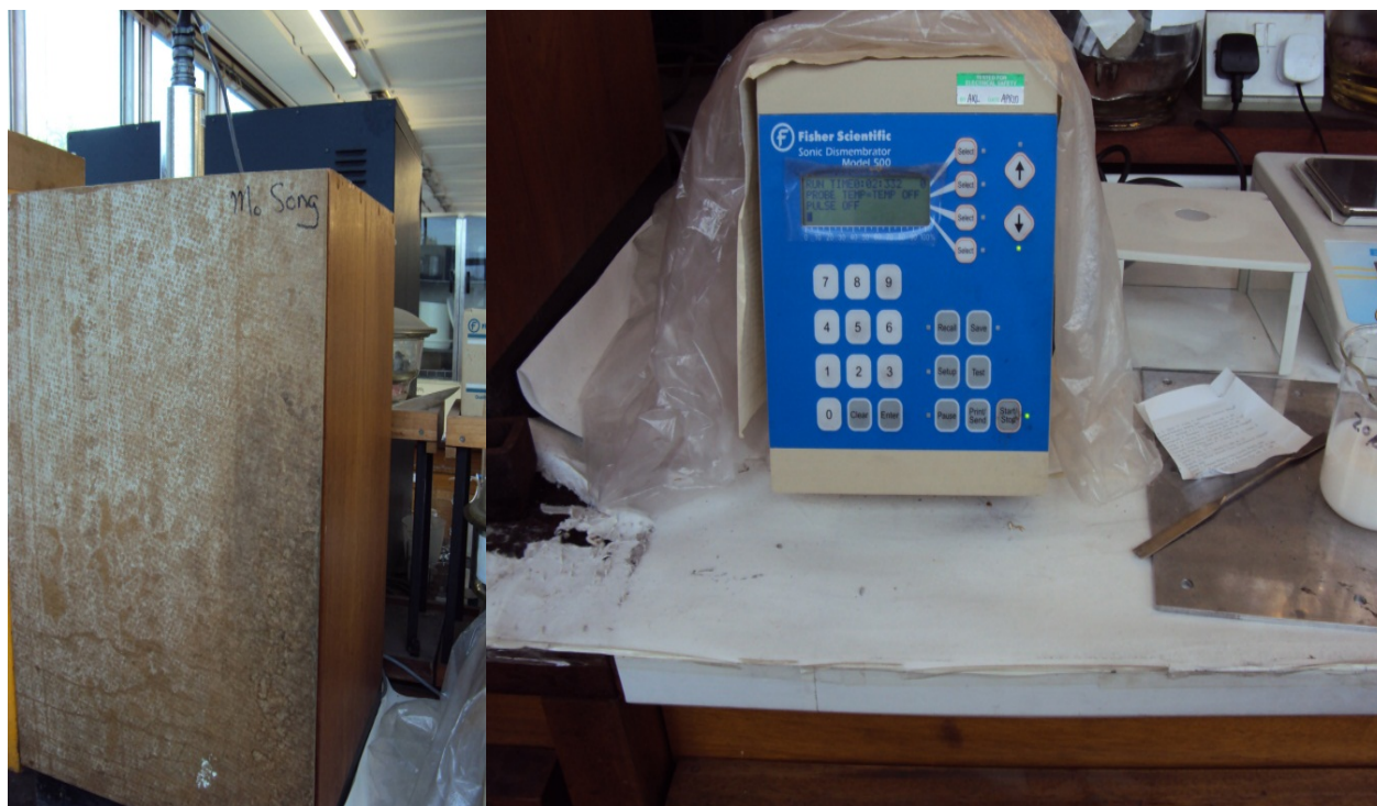
Fig.3.1: Ultrasonic dismembrator with disruptor horn cabinet
