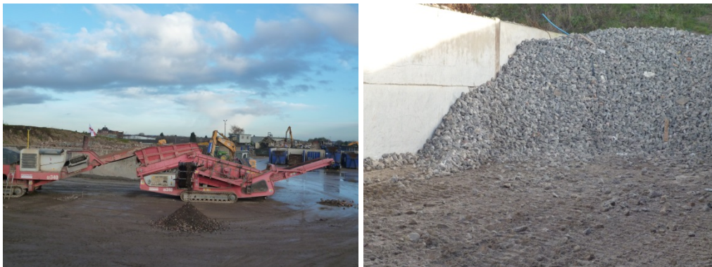
Figure 3 Stages of concrete demolition and recycling with the potential to cause dust release
