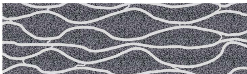
Figure 0.2 Schematic structure of PEDOT:PSS (after ref. [92])
