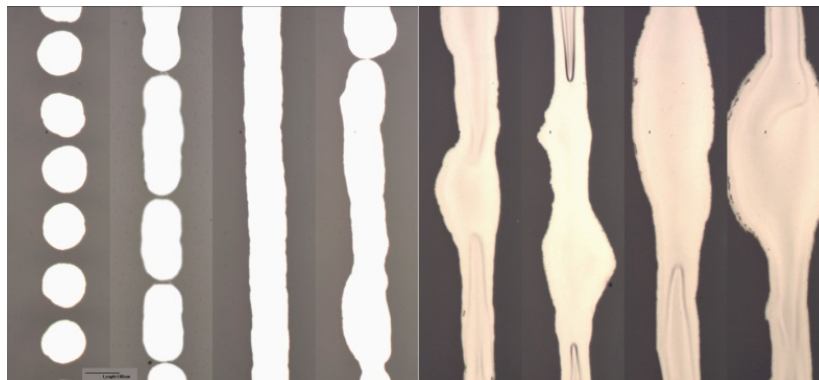
Figure 0.28 Printed silver tracks with different dot spacing values (from left to right: 170 \mu\text{m} , 125 \mu\text{m} , 110 \mu\text{m} , 100 \mu\text{m} , 80 \mu\text{m} , 70 \mu\text{m} , 60 \mu\text{m} and 50 \mu\text{m} . The average dot diameter is approximately 150 \mu\text{m} )
