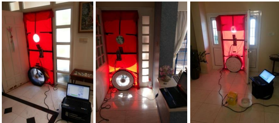
Figure 3-10 Photo of the Blow-Door equipment (left to right SD1, SD2, and SD4)
