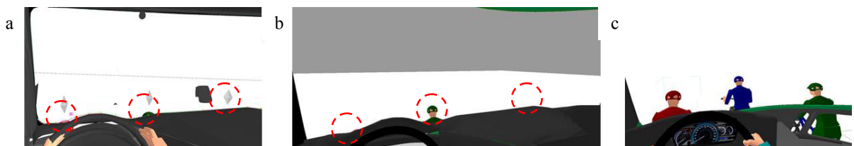
Fig. 6. (a) Driver's eye view of cyclist visibility for the DAF XF baseline vehicle (b) FKA concept (c) FKA concept iteration 2.
