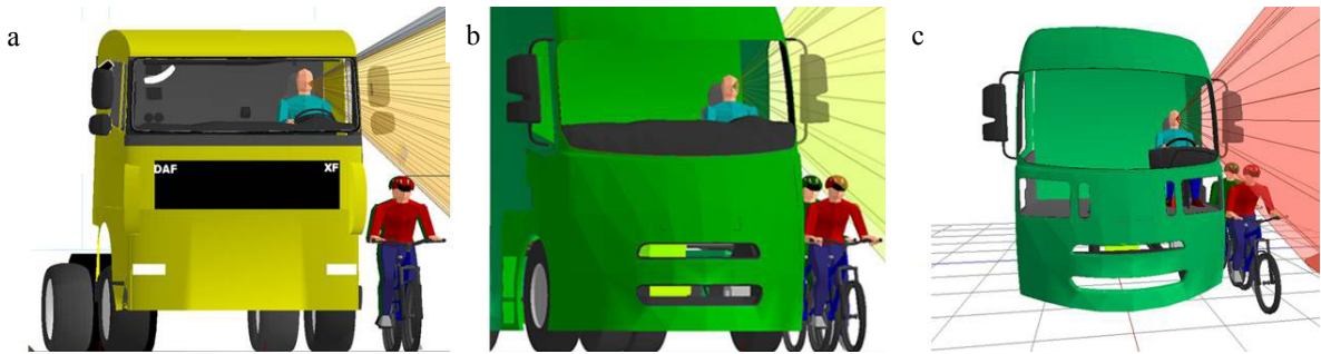
Fig. 9. (a) Cyclist visibility to the driver's side of the DAF XF baseline vehicle (b) FKA concept (c) FKA concept iteration 2.
