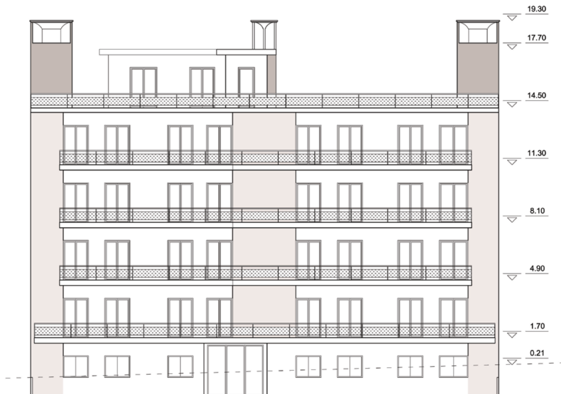
Figure 4.19 Southeast elevation of the building under investigation, showing the three wind-catchers in the core spaces (dimensions in metres, nts)
