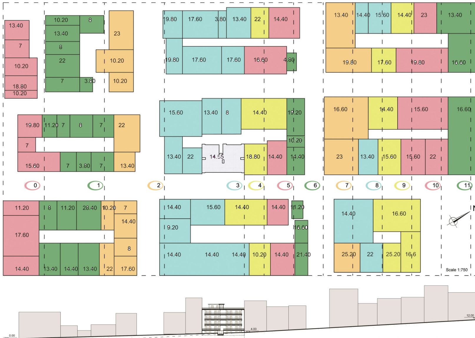
Figure 4.8 Plan view of the site showing building heights in metres, with different colours the 1-metre contours, and a front elevation
