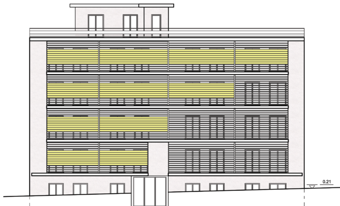
Figure 4.25 A southeast elevation showing the operation of the shading system at each balcony in relation to solar shade.
