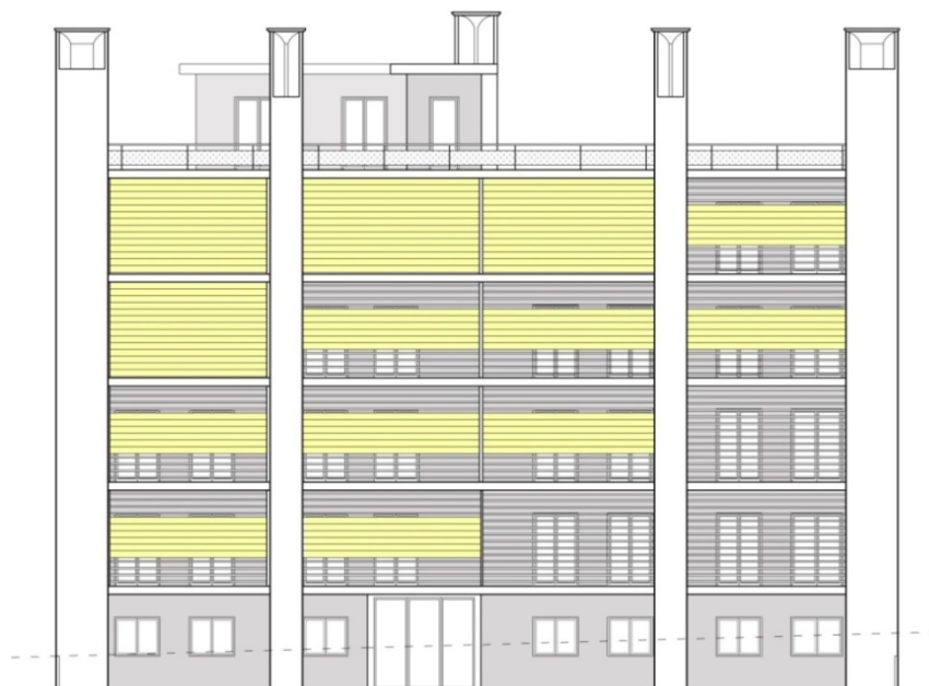
Figure 4.28 Southeast elevation of the building under investigation, showing the operation of the shading system on each balcony and the façade wind-catchers, nts
