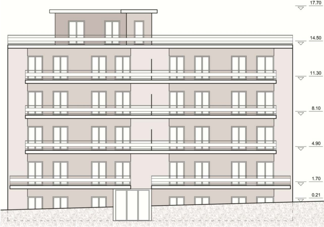
Figure 4.3 East Elevation, CAD drawing of the building studied by author (metres, nts)
