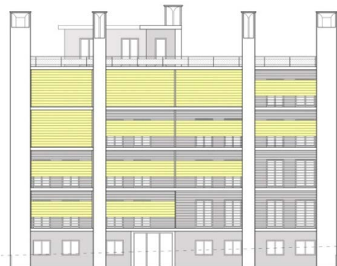
Figure 7.54 South-east elevation of the building studied, showing the operation of the shading system in response to solar radiation, and the wind-catchers
