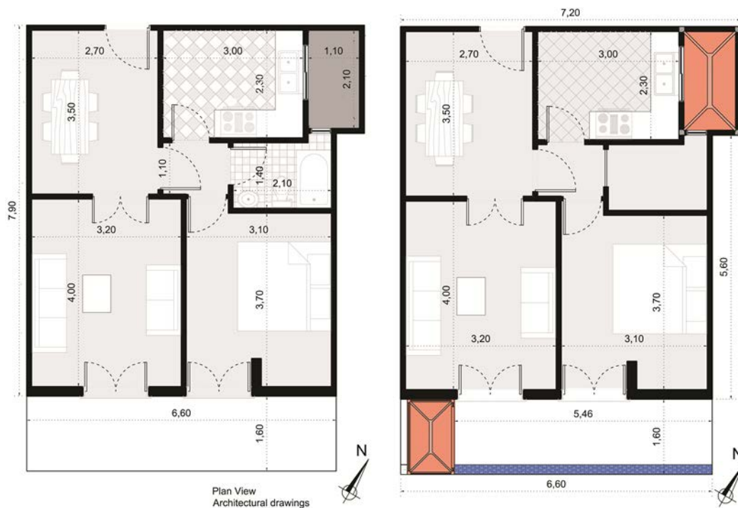
Figure 7.55 Plan view (left) and updated plan view (right) of the apartment studied showing the wind-catcher, the façade wind-catcher and optimization the dynamic façade
