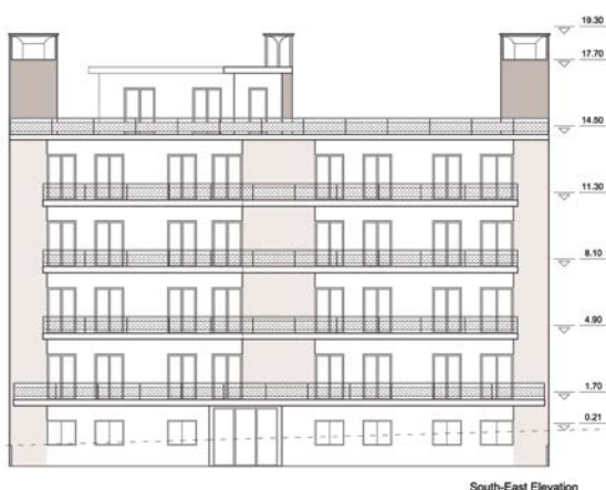
Figure 7.47 South-east elevation of the building under investigation, showing the three wind-catchers at the core spaces
