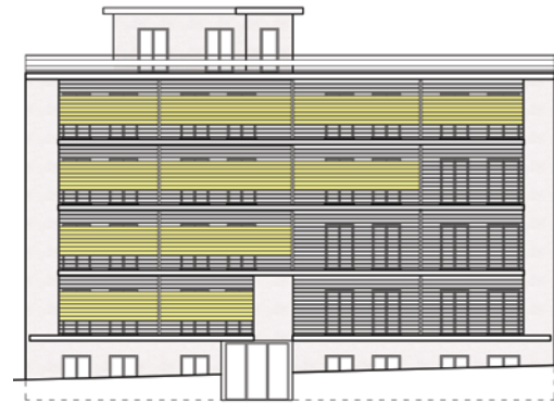
Figure 7.51 South-east elevation of the building studied, showing the operation of the shading system in response to solar shade.
