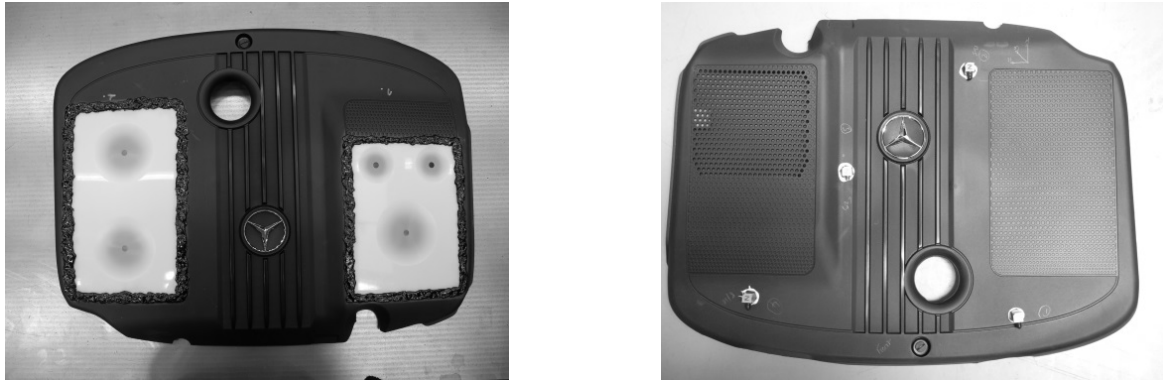
Fig. 11 - ABH engine cover –top view and location of accelerometers on reference engine cover
