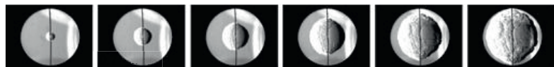
Fig.5 H 2 -Air flame at Φ=0.6, 298K and 1bar. Measured flame radii are: 5.8, 12.1, 17.8, 23.9, 30.0 and 35.0mm
