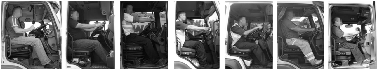
Figure 5. The variety of driver postures exhibited by drivers with a 4th%ile to 99th%ile stature range using UK anthropometric data (ADULTDATA 1998)
