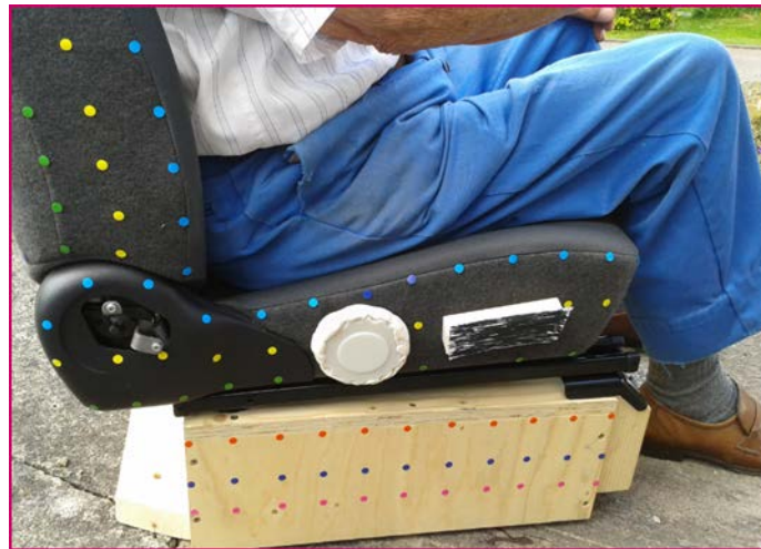
Figure 69: Seat recliner and the seat lifter (manual - dial and lever type adjustments)
