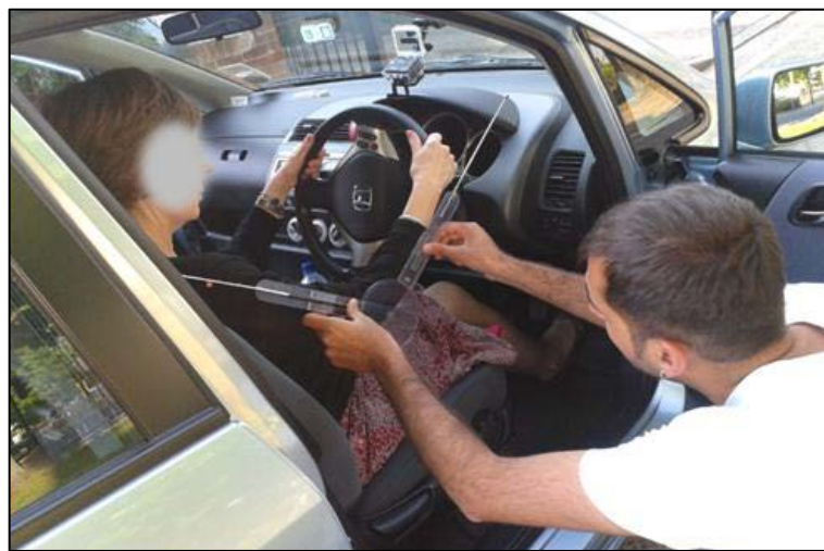
Figure 30: Measuring static driving posture with extendable goniometer
