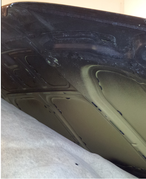
Fig. 6. Illustration of a typical automotive panel (bonnet shown) with holes for weight saving and attachment of the heavy trim liner (bottom of the photo). Automotive bulkheads typically have access holes for cables and heating ducts. Typical solutions for noise and vibration include attachment of viscoelastic damping layers.
