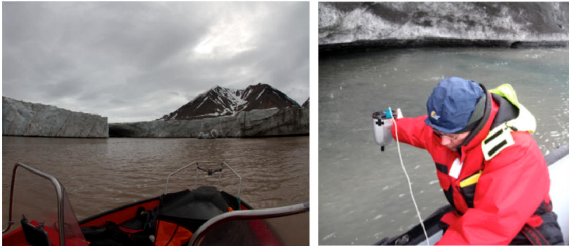
Figure 4.2: Left: A small boat was used to access the waters at the ice front of Kronebreen, Svalbard. Right: Hand held spectroradiometer was used to measure spectral reflectance of the surface water (Photo depicts same instrument and technique, but is located in Iceland).
