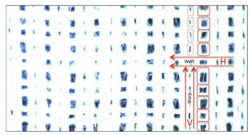
Figure 71: Woven PET fabric structure showing spacing of warp yarns and weft yarns (x5 mag.)
