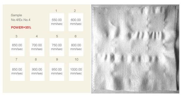
Figure 40: Configuration of laser parameters explored using the CO2 10W Synrad laser marker (left); and the resulting woven polyester woven fabric sample (right)
