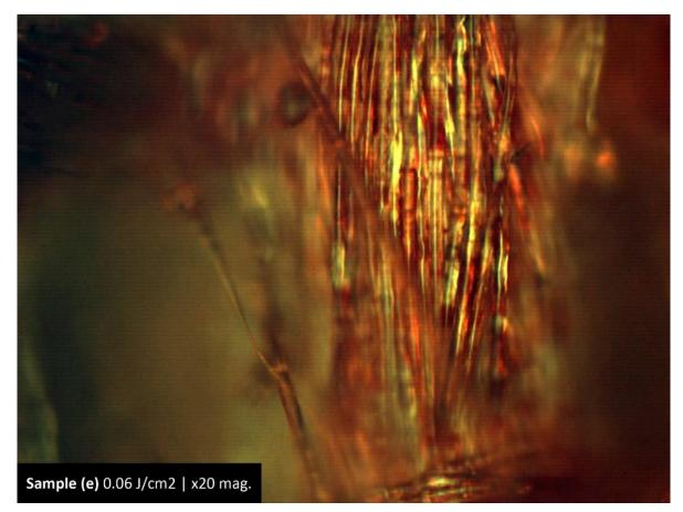
Figure 154: Sample (e): showing sufficient coloration without significant damage when processed with 0.06 J/cm2 energy density.
