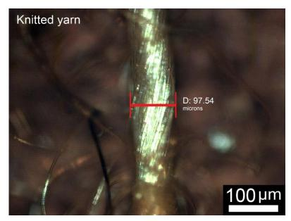
Figure 83: Micrograph of individual yarn taken from knitted PET fabric (x10.100 magnification)
