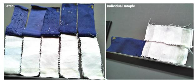
Figure 118: Fabrics assessed inside light cabinet for wash fastness by batch and per specimen
