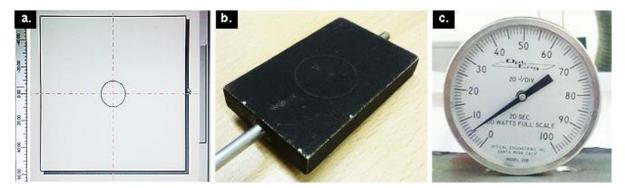
Figure 42: Computer screen/central spot (a); 10-100W Power meter probe (b); and gauge (c)
