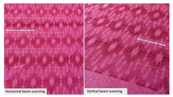
Figure 62: Visible overlapping 'streaking' effect as a result of beam overlap during scanning
