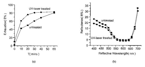
Figure 18 (Left): Exhaustion rate of laser treated and untreated dyed polyester samples (Lau et al. 1997, p. 526) Figure 19 (Right): Colour reflectance of laser treated and untreated dyed polyester samples (ibid)
