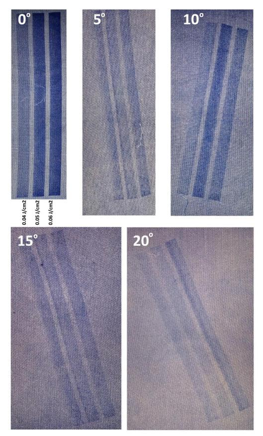
Figure 160: Axis experiments with woven PET samples laser modified at 0°, 5°, 10°, 15° and 20°
