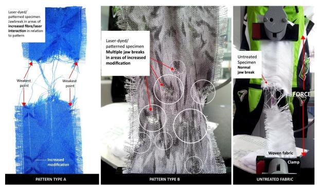
Figure 127: Tensile strength tests showing jaw break: Pattern Type A, B and Untreated specimen
