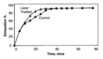
Figure 22: Exhaustion rate in acid bath - laser treated and control PA fabric samples (Shahidi et al. 2013, p.43)
