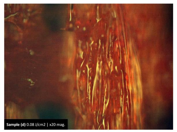
Figure 153: Sample (d): showing damaged fibres when processed with 0.08 J/cm2 energy density.
