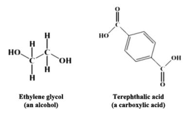
Figure 3: Starting compounds for the manufacture of PET fibre (Shamey and Shim 2011, p. 98)
