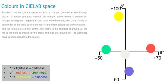
Figure 103: CIELAB (CIE L\*a\*b\*) colour model, SDC, 2013
