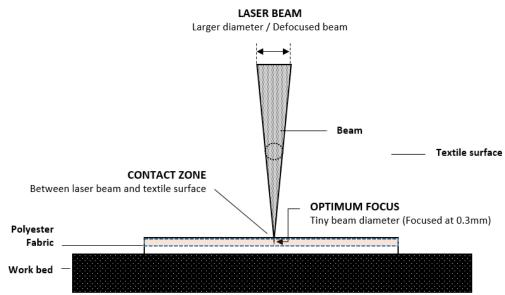
Figure 36: Fibre-laser interaction
