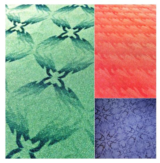
Figure 60: FLD processed woven PET fabrics demonstrating different pattern types explored
