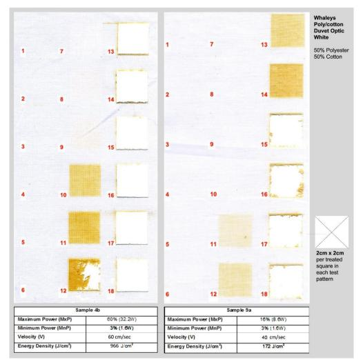
Figure 49: Laser modified poly/cotton samples (4b) and (9a) with a 18 greyscale test pattern
