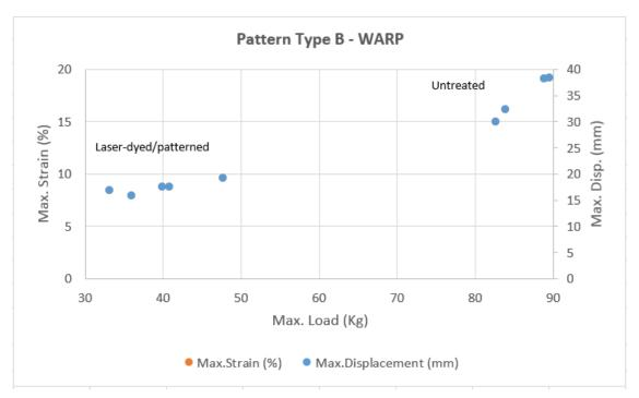
Figure 126: Tensile Strength results graph: WARP - Pattern Type B and Untreated fabric
