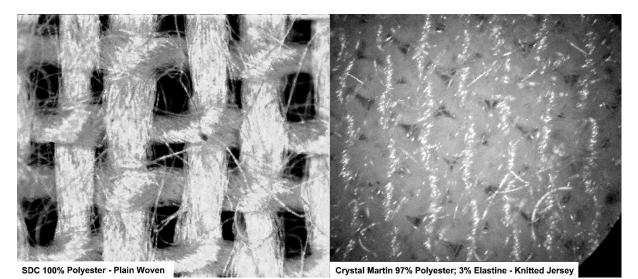
Figure 56: Structure of untreated woven (a) and knitted (b) polyester at 10.100x magnification
