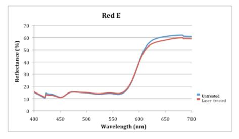
Figure 101: Reflectance for Batch 5: Red E - Laser-dyed fabrics: GS: 70% and GS: 100% (Red E)
