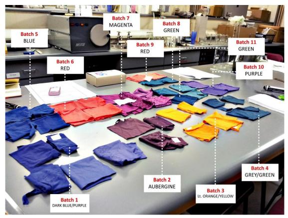
Figure 115: Wash fastness samples (x39 specimens) for testing arranged into batches by shade
