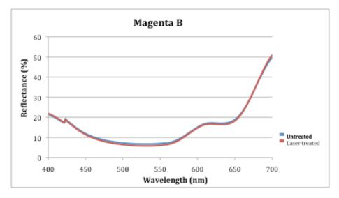
Figure 97: Reflectance/Batch 2: Magenta - Laser treated and untreated fabrics: GS: 70% (Magenta B)
