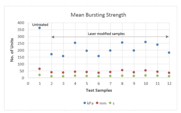
Figure 134: Bursting strength results graph
