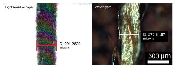
Figure 79: Laser beam scan with Synrad 60W Laser (left), Individual woven polyester yarn (right), x10.100 magnification
