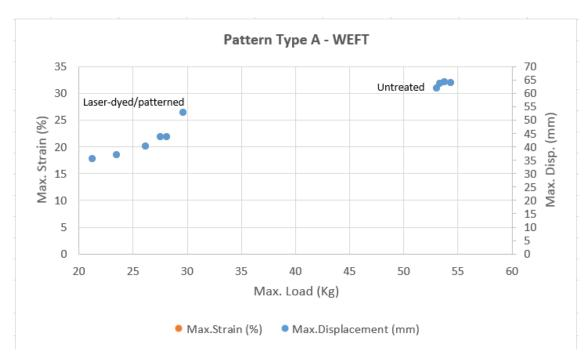
Figure 125: Tensile Strength results graph: WEFT - Pattern Type A and Untreated fabric
