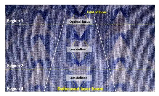
Figure 59: FLD processed woven PET sample showing reduced sharpness due to defocused beam
