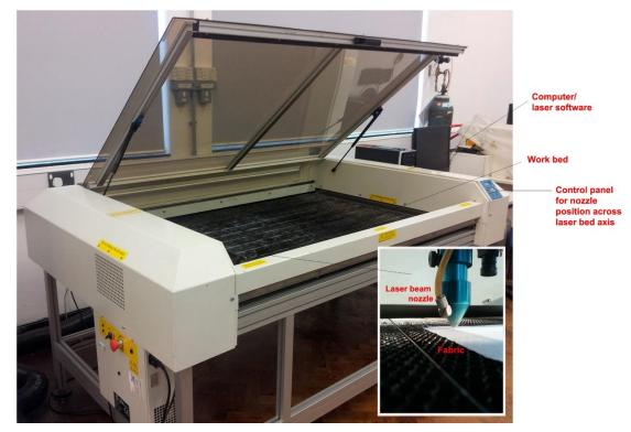
Figure 47: 58W CO2 Laser bed system
