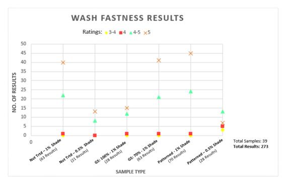
Figure 120: Wash fastness test results graph
