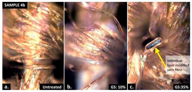
Figure 50: Laser treated woven poly/cotton (50%/50%) sample (4b) viewed at x20 magnification
