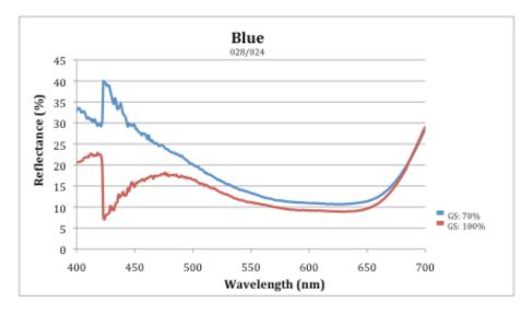
Figure 96: Reflectance/Batch 1: Blue - Laser-dyed fabrics: GS: 70% and GS: 100% (Blue)
