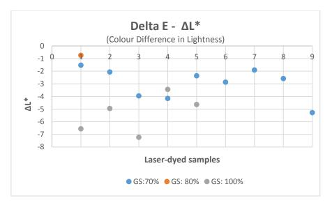
Figure 106: Delta E Colour difference: Lightness results ( $\Delta L^*$ )
