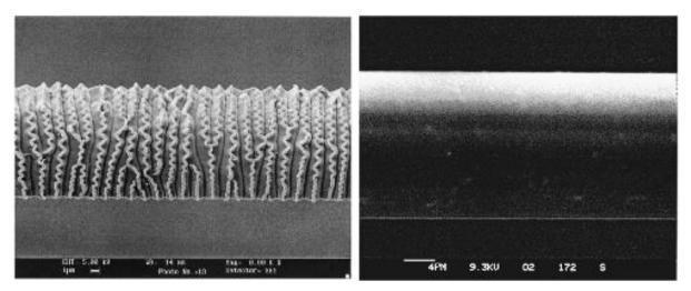
Figure 14: (Left) Surface structure of laser treated polyester under high fluence (Kan 2008b, p.115) Figure 15: (Right) Surface structure of untreated polyester (Kan 2008b, p.115)
