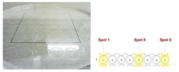
b. (Left) Orientation of burn print: laser spots fired on to acrylic specimen;
