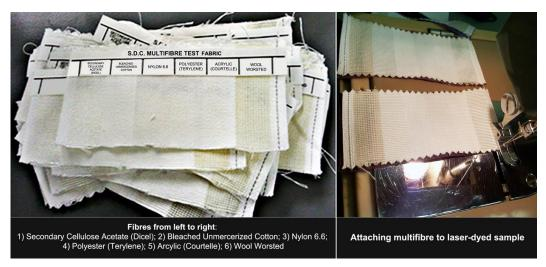
Figure 116: SDC Multifibre DW; Prepared for wash fastness tests
