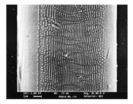
Figure 17: Surface structure of laser treated polyester under low fluence (Kan 2008b, p.116)
