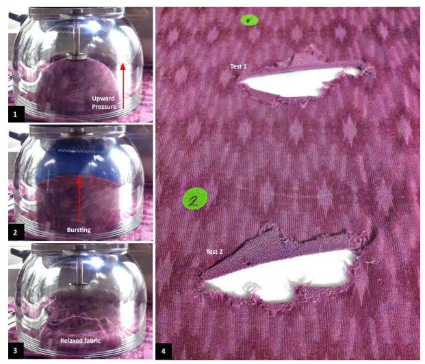
1. Laser-dyed textile sample subject to a surge of air pressure during test; 2. Bursting threshold - fibre breakage, 3. Relaxed fabric after testing; 4. Tested sample
