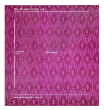
Figure 64: FLD patterned fabric sample showing inertia leading to darker edges (woven PET)
