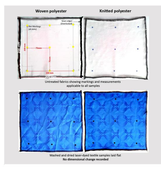
Figure 135: Samples tested for dimensional stability
