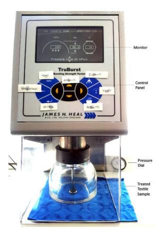
Figure 132: Bursting Strength Tester Machine
