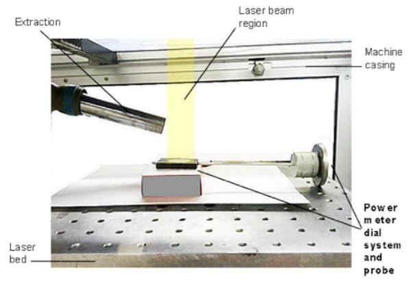
Figure 41: Measuring power output of CO2 Synrad 10W laser marker
