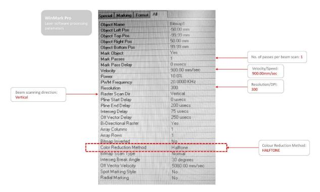
Figure 67: WinMark Pro laser software processing parameters showing: 'Halftone' colour reduction mode
