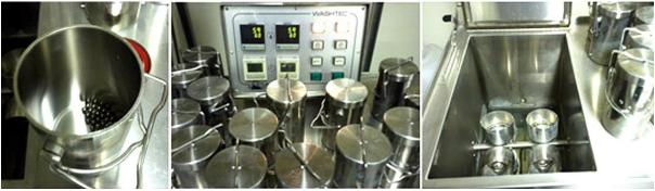
Figure 117: Individual beakers and Washtech machine
