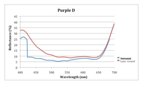
Figure 100: Reflectance/Batch 4: Purple - Laser treated and untreated fabrics: GS: 70% (Purple D)
