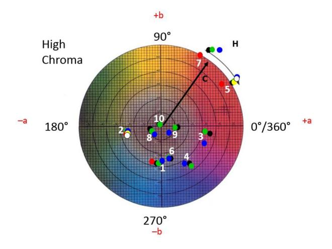
Figure 105: Fabric samples quantified in L\*C\*H\* lab space
