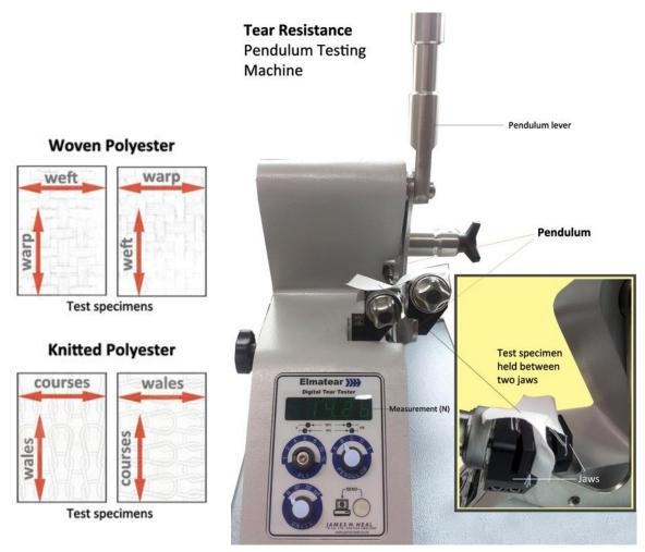
Figure 128: Tear Resistance specimens - woven and knitted polyester fabrics (Left) Figure 129: Tear Resistance Pendulum Testing Machine; Inset: Test Specimen (Right)
