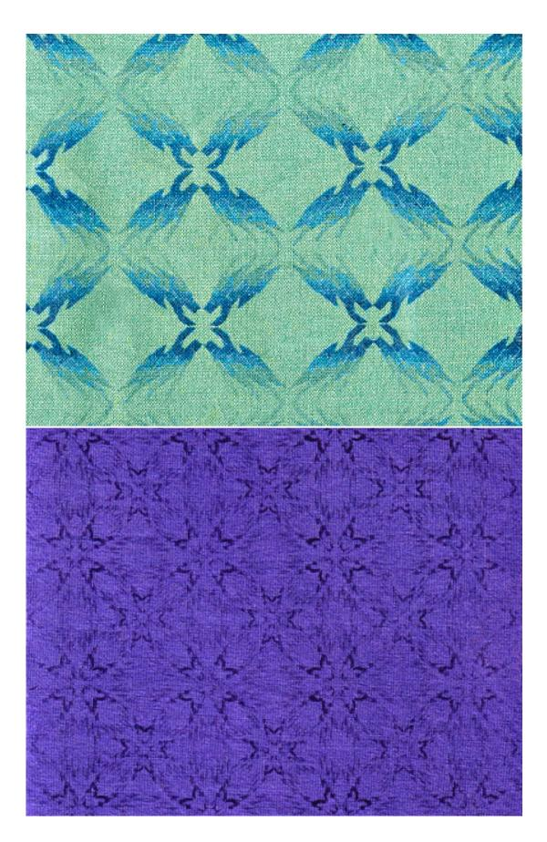
Figure 141: Laser-dyed woven (above) and knitted (below) PET textile samples generated using a raster approach: Engineered repeat patterns
