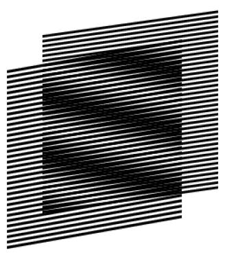
Figure 76: Moiré pattern caused by identical linear patterns overlaying at a slight angle (bowiestie.wordpress.com 2010)
