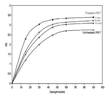
Figure 20: Dyeability of CW laser treated PET fabric at different exposure times (Kamel et al. 2012, p. 4)
