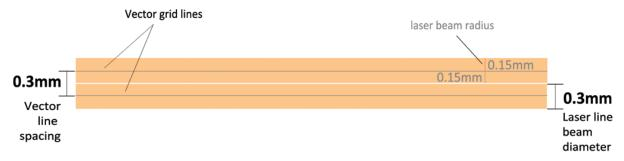
Figure 89: Diagram showing the position of a 0.3mm laser line vector grid
