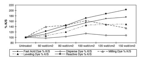
Figure 23: %KS of treated and untreated fabrics (Bahtiyari 2011, p.115)
