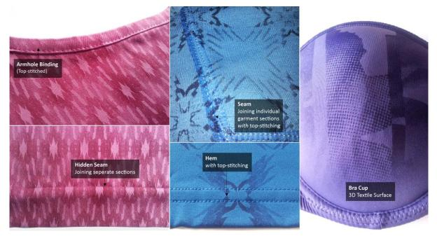
Figure 145: Laser-dyed finished garments and 3D clothing - construction and surface
