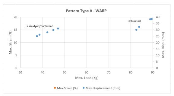
Figure 124: Tensile Strength results graph: WARP - Pattern Type A and Untreated fabric
