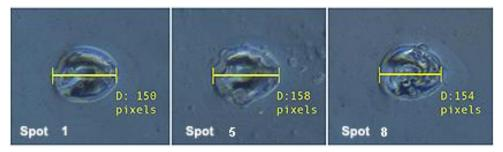
d. Micrographs of acrylic burn print (x10.100) showing the number of pixels/diameter per spot
