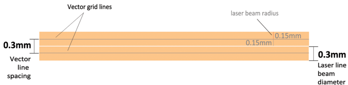
Figure 9: Diagram showing the position of a 0.3mm laser line vector grid
