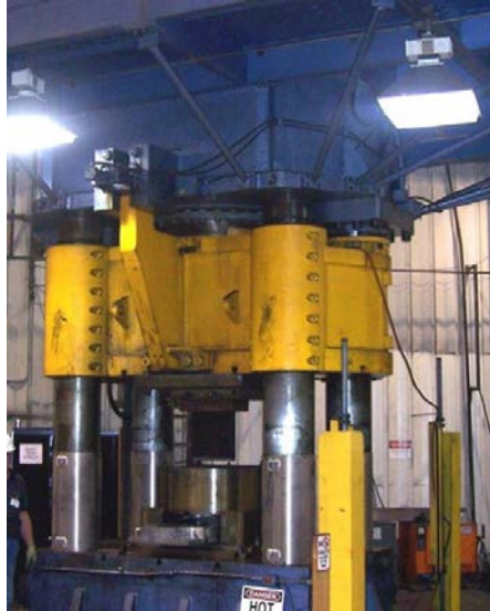
Fig. 2.33 Production ECAP die with 4000 tonnes press capacity [112].
