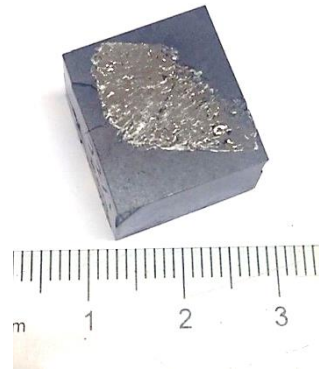
Fig. 6. 1 Ti-15V-3Cr-3Al-3Sn chips pressed at room temperature without back-pressure.
