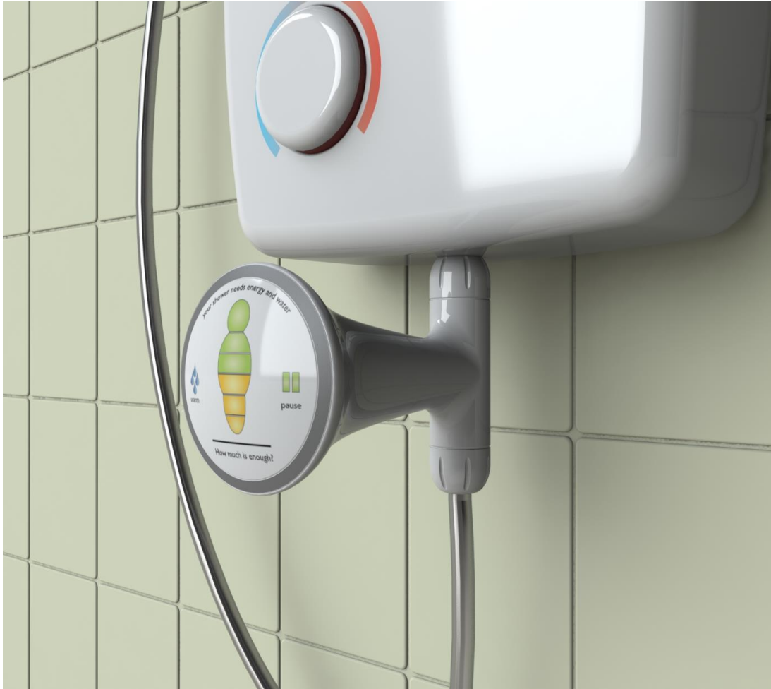
Figure 9-5. Revised Enuf concept with in-line turbine power.
