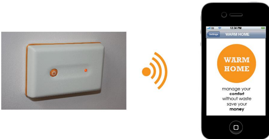
Figure 6-8. Warm Home system showing 'dumb' wall-mounted unit and digital control interface.
