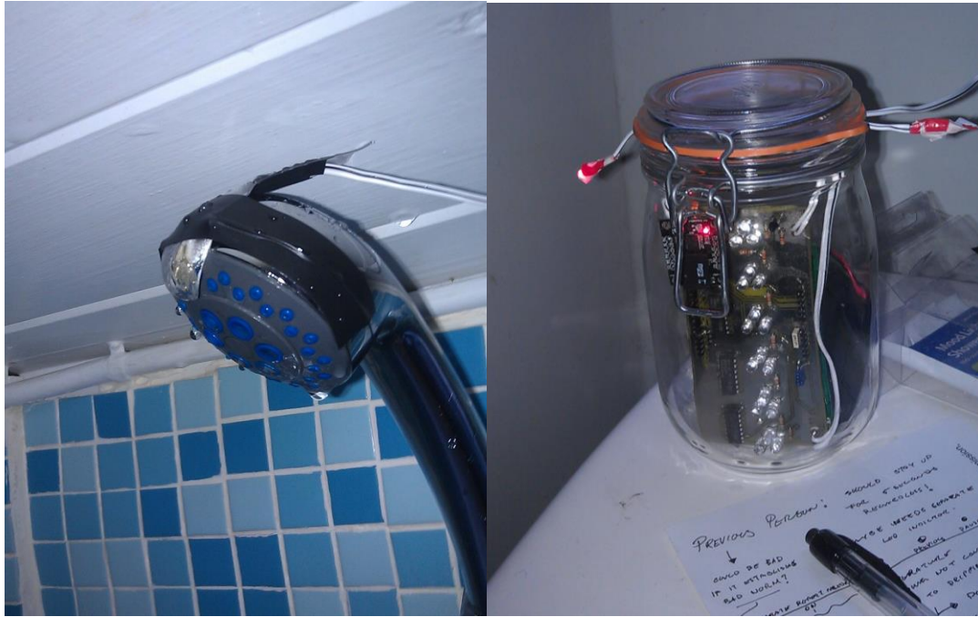
Figure 6-30. Early testing of prototype with improvised water-proof housing.
