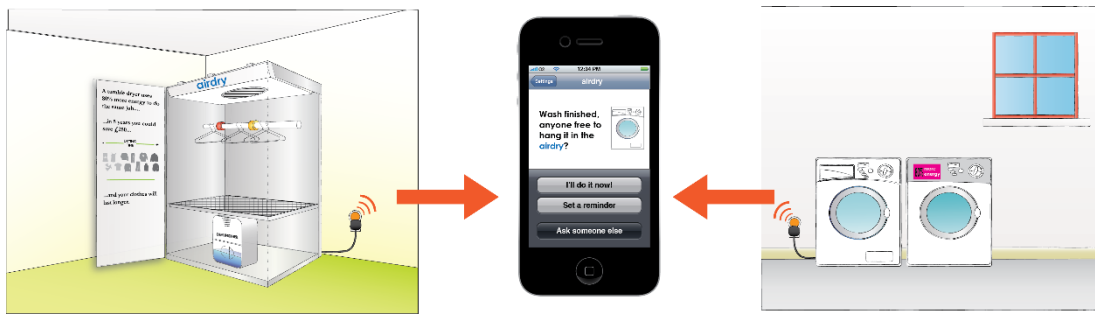
Figure 6-16. AirDry energy monitor network.
