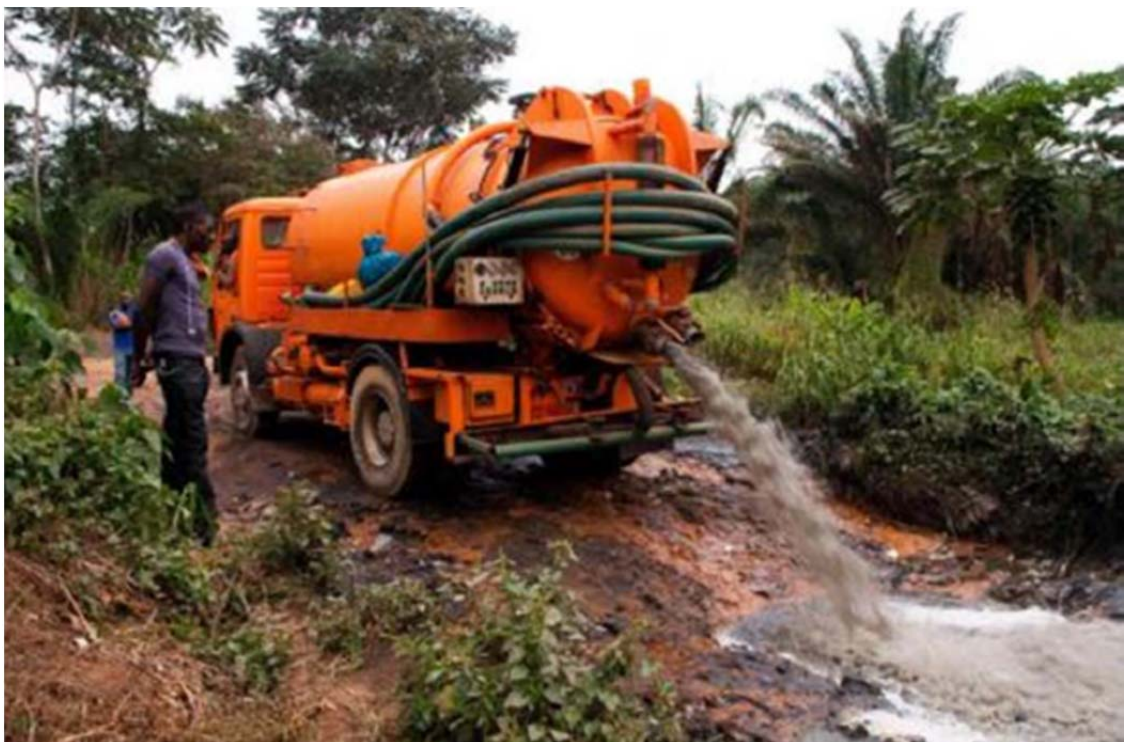
Fig.1.3 Emptying trucks to dispose of HBW slurry [adapted from (19)]
