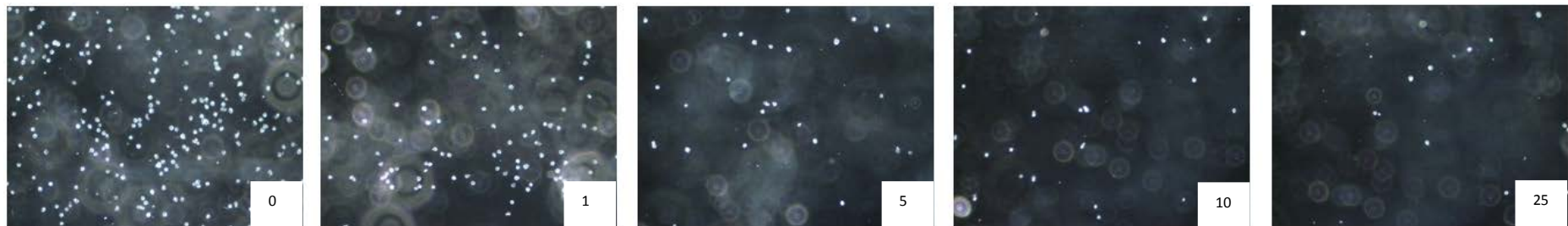
Figure 2-23. Microscope images of HLA-A2 cells (CD20-) incubated with IgG antibody, introduced into the flow tubes and incubated for 30 minutes prior to washing over shear stresses of 0, 1, 5, 10 and 25 dynes/cm 2 applied sequentially for 3 minute intervals each (control study for non-specific cell adhesion).
