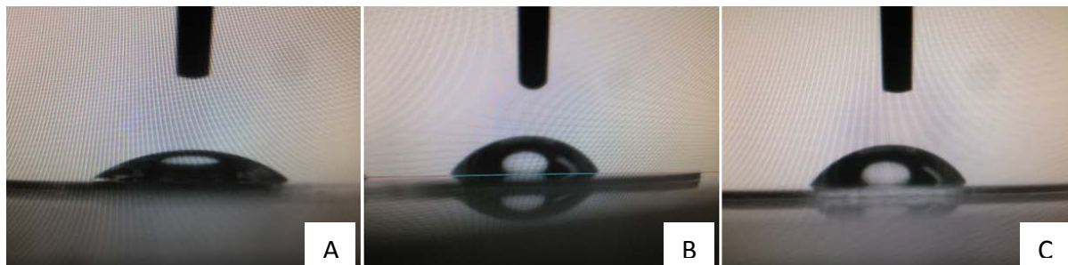
Figure 2-8. Contact angles for cleaned glass (A); APTES-treated glass (B) and APTES-glass treated with glutaraldehyde (C).
