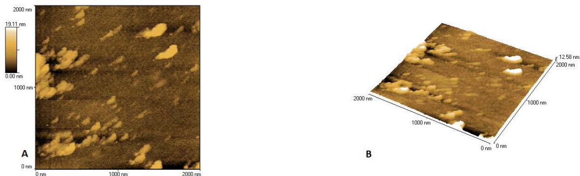
Figure 2-12. AFM images for aldehyde-treated aminated glass (2 x 2 \mu\text{m} ) in a two-dimensional display (A) and a three-dimensional display.
