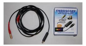
Figure 2. Underwater endoscope camera (resolution: 640 × 480 pixels; price July 2013: £25).
