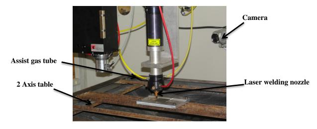
Figure 4-1 Experimental setup used for laser welding
