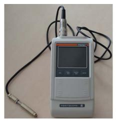
Figure 3-9 Determination of the ferrite content in the weld seam area using the FERITSCOPE
