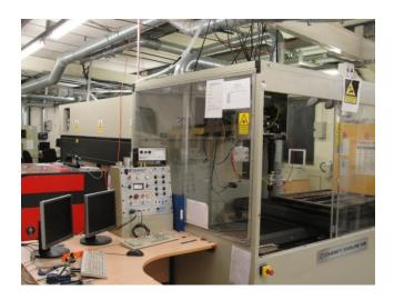
Figure 3-3 1.2kW Carbon dioxide (CO<sub>2</sub>) coherent S48 laser systems
