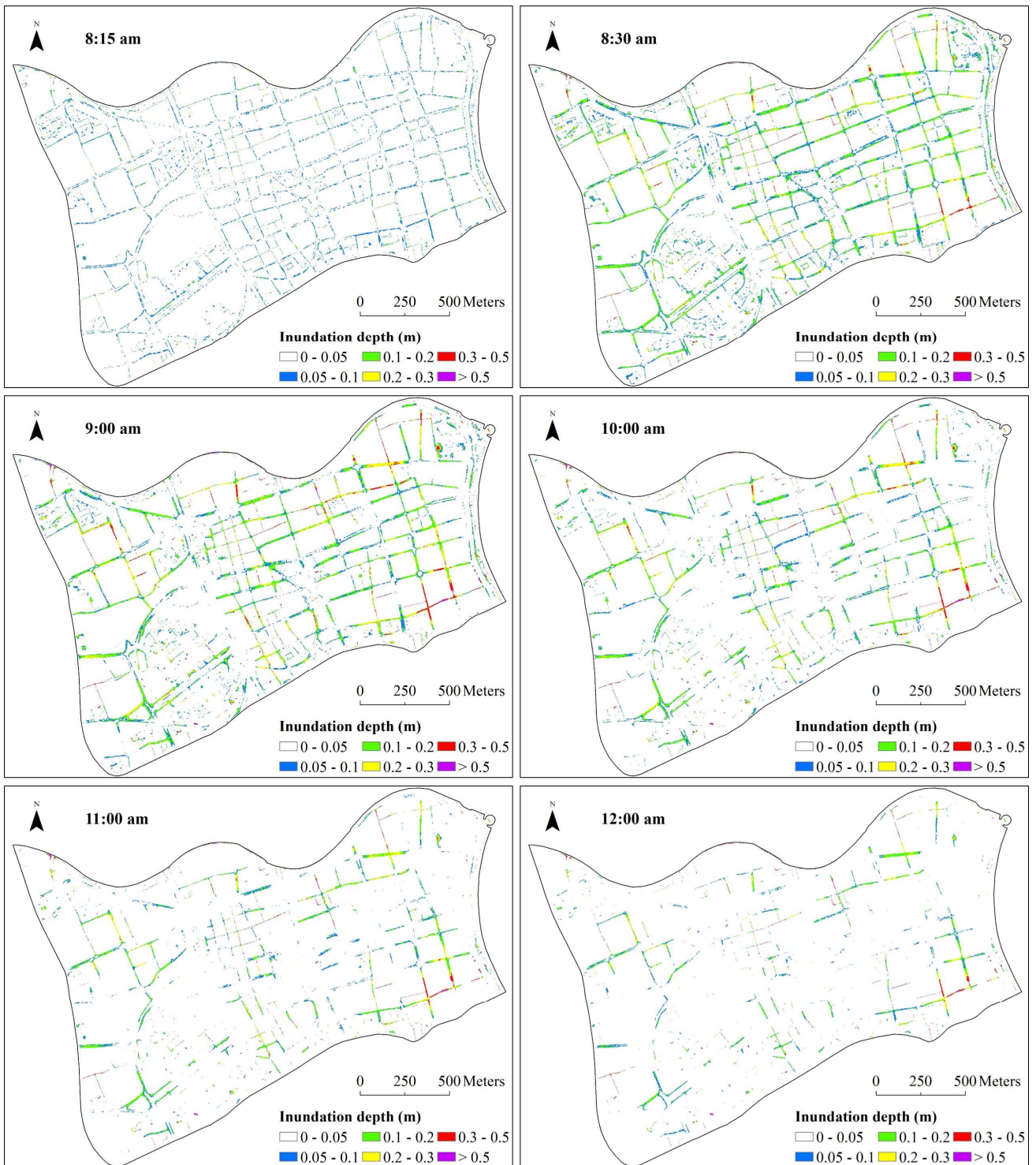
Fig.4 Time series of predicted inundation depth for the August 2011 pluvial flood event.
