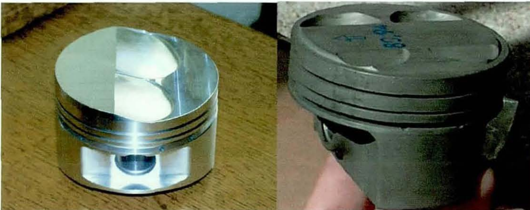
Figure 2.2(a): Piston skirt design variation according to application (shown on the left is a full skirt piston and on the right short skirt)
