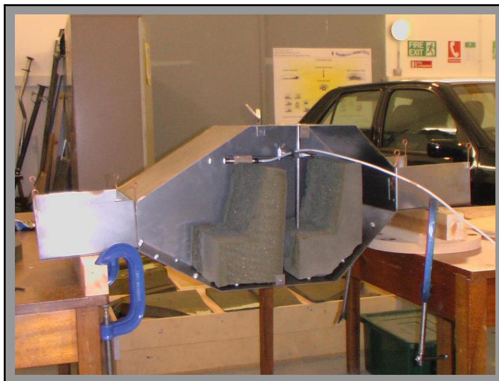
Fig. 8. View of the interior of the whole model with the inserted foam seats.
