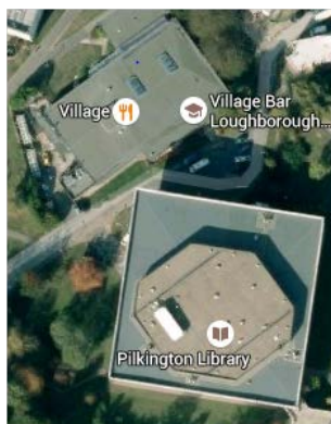
Figure 2: Shade (grey) on roofs of Pilkington Library (square building) and Village Restaurant, at foot of hill, West Campus, Loughborough University, noon 22 December 2015
