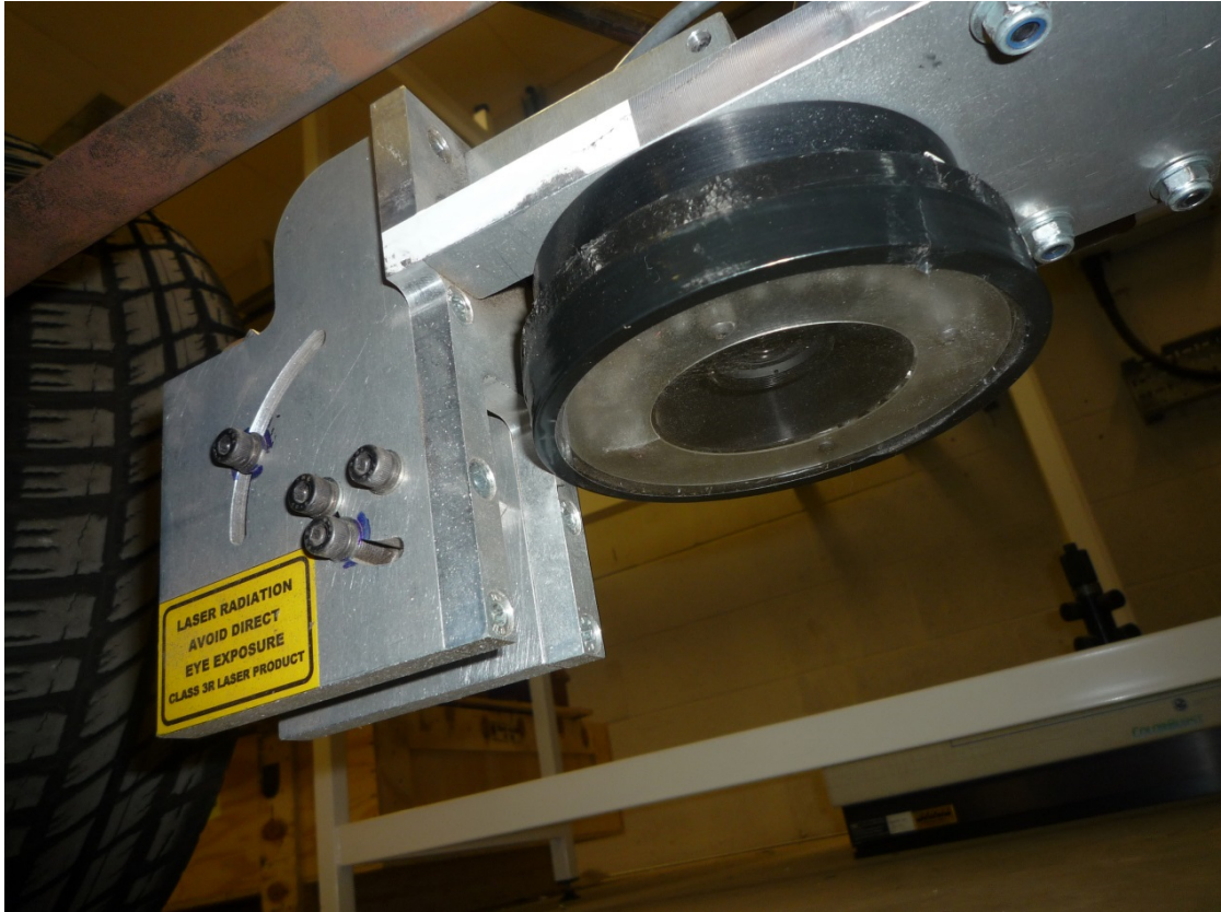
Figure 7. An optical displacement sensor (ODS) used as part of a system to determine vehicle trajectory and body motion.
