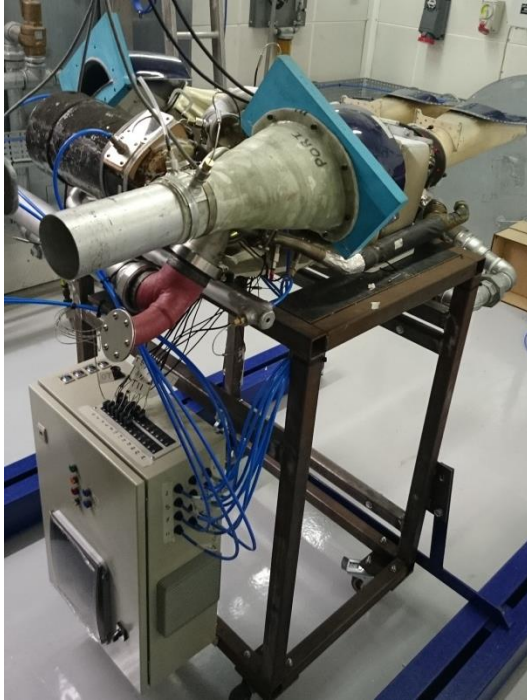
Figure 2. ECS Test Stand Installation. (a) shows the front of the system; with ram air inlet and control / DAQ cabinet visible. (b) shows the rear of the system; with bleed air inlet, ram air exhaust and heater control cabinet visible.
