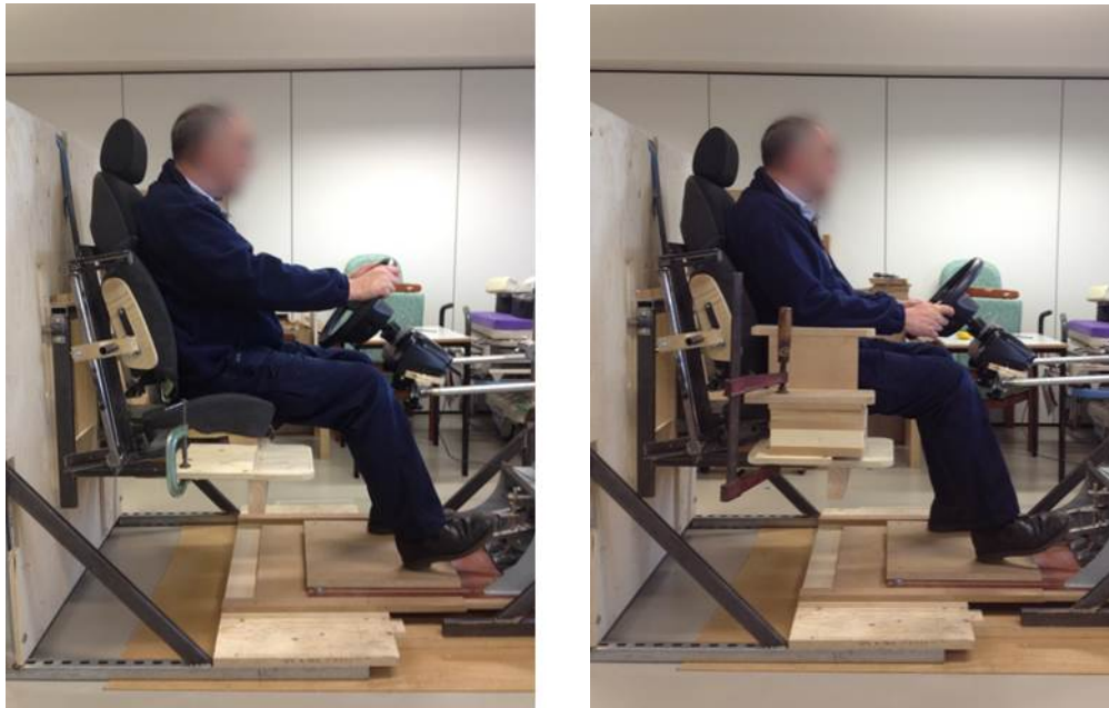
Figure 4.3. AM87 male participant in their optimised elevated driving posture; left to right, side profile without armrest and with armrest.
