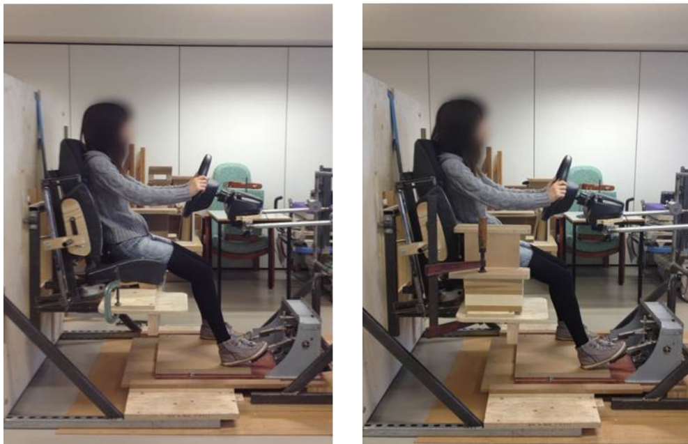
Figure 4.2. JF07 female participant in their optimised elevated driving posture; left to right, side profile without armrest and with armrest.
