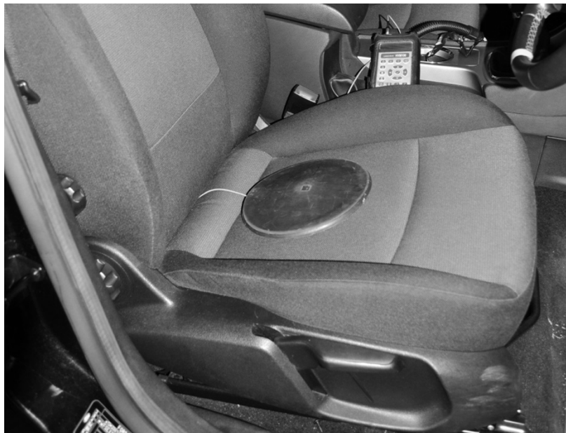
Figure 3.10. Adjusting seat-system characteristics using the Larson Davis HVM-100 with tri-axial seat pad accelerometer (image taken from Mansfield, 2005).
