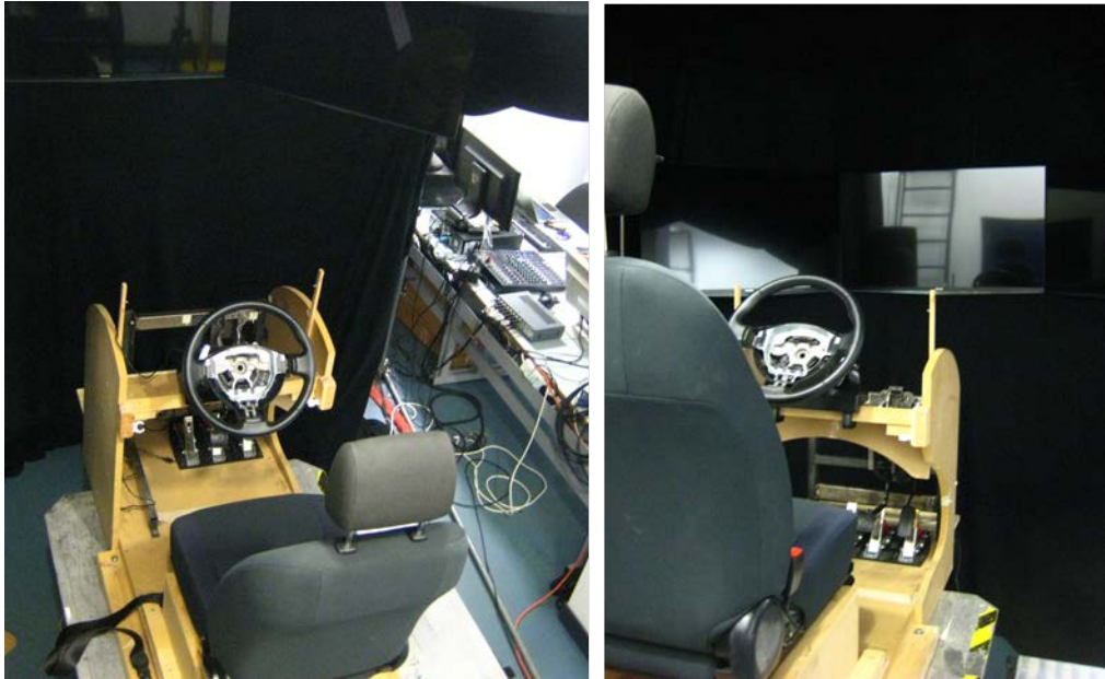
Figure 5.4. Blackout environment in development (left) and completed, surrounding the test area (right).
