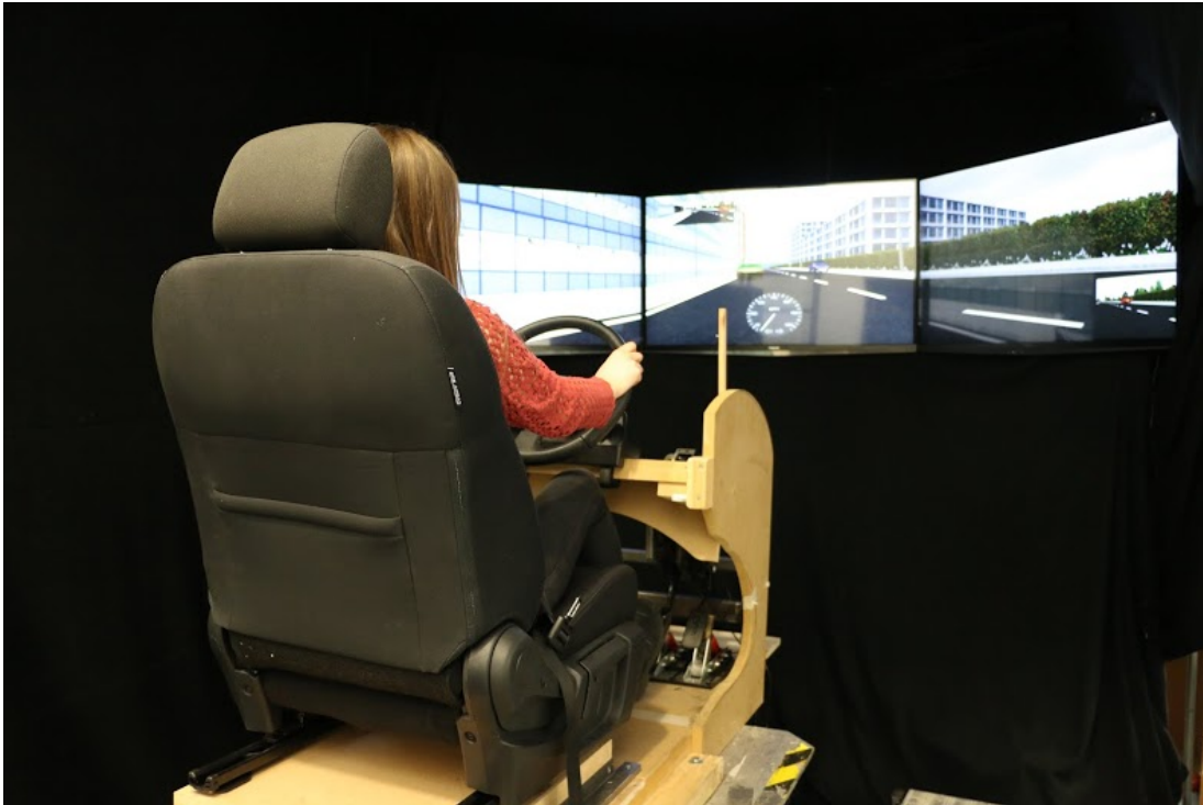
Figure 3.11. Three-screen XPDS driving simulator set-up in the vehicle laboratory environment in front of the vibration platform and mounted driving rig.
