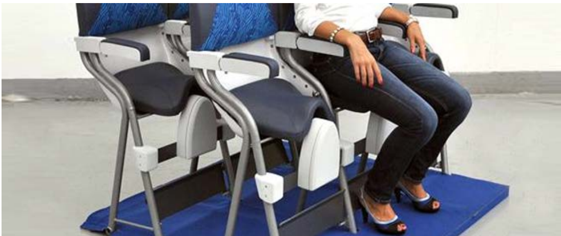
Figure 7.6. AvioInteriors concept aircraft seat design ‘SkyRider’ (image taken from Wired Online article, 2015).
