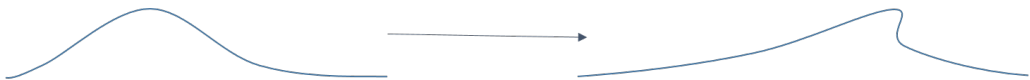
Figure 1.1: Time evolution of u_t = uu_x with a Gaussian initial profile. The profile becomes steeper, and breaks down in finite time.
