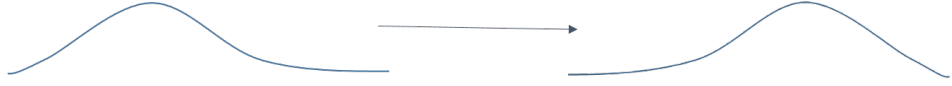
Figure 1.2: Time evolution of u_t = cu_x with a Gaussian initial profile. The initial profile translates with finite speed c without changing its shape.
