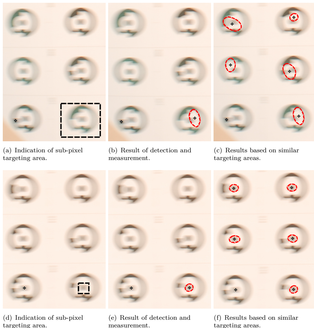
Figure 3.6: Semi-automatic target detection and measurement on image with 1.03 mm camera displacement.
