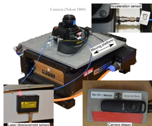
Figure 2. Shaker table with camera mounted on it.
