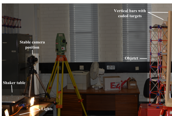
(c) Photo of laboratory set up.
