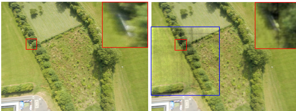
(a) Enhanced image using unsharp mask method. (b) Enhanced image using frequency transfer method. In blue enhanced area.
