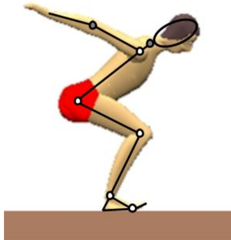
Figure 17. 8-segment model of vertical jumping (grey circles angle-driven joints; white circles torque driven).
