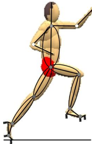
Figure 13. 13-segment model of triple jump takeoffs.
