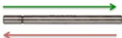
Figure 13 An image of a thermal desorption tube showing the sampling and conditioning flow directions flow (green and red arrows respectively)
