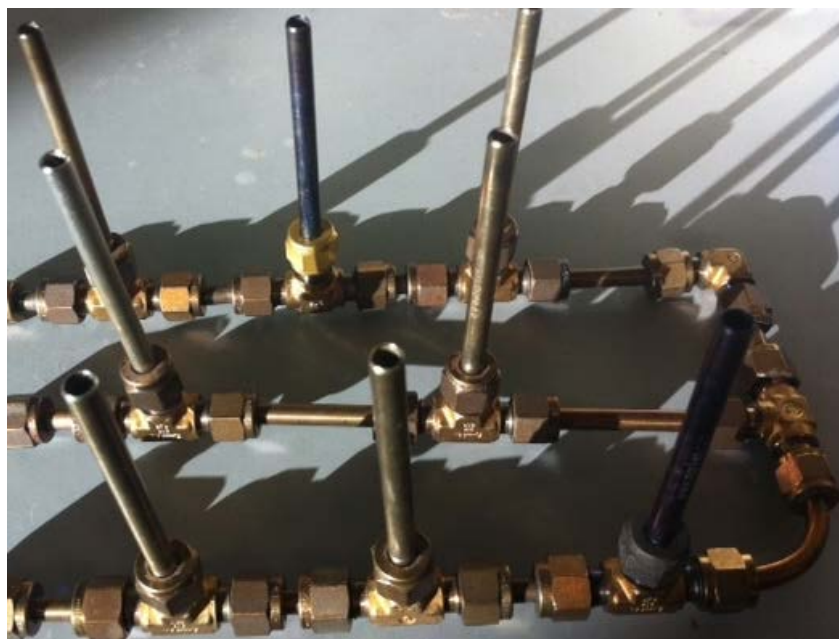
Figure 14 The adsorbent tube conditioning manifold was installed into a GC oven where up to eight adsorbent sample tubes were processed at the same time.
