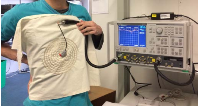
Fig. 5. Measured set up for the embroidered spiral antenna on-body measurement
