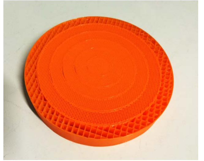
Fig. 3 3D-printed flat lens
