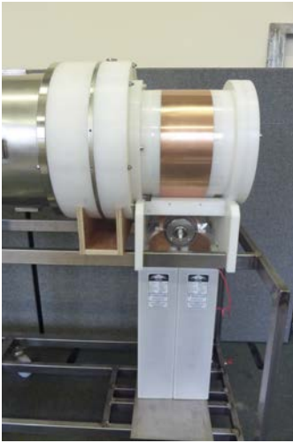
Fig. 8. Tesla transformer secondary winding
