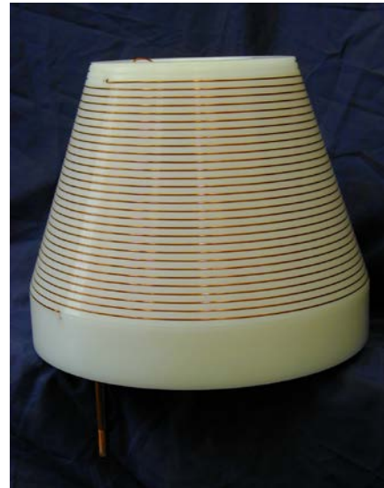
Fig. 3. Tesla transformer secondary winding
