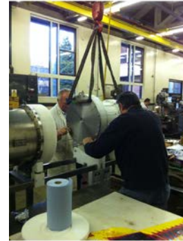
Fig. 10. Aspects from manufacturing and assembly (a) outer and intermediate electrodes partially assembled (b) inner electrode ready for mounting (c) attaching the Tesla to the B-PFL
