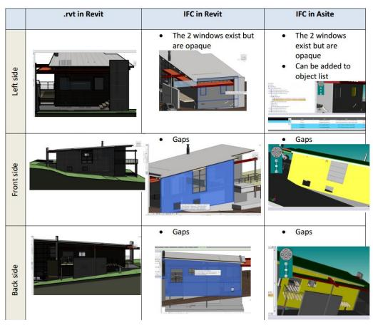
Figure 23 Issues with windows elements in Revit to IFC conversions
