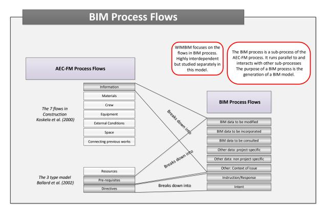
Figure 353 AEC-FM Process Flows and BIM Process Flows
