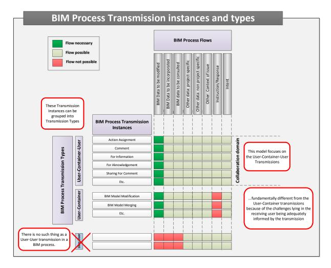
Figure 37 BIM Process Transmissions: Main categories and relation to BIM Process Flows.
