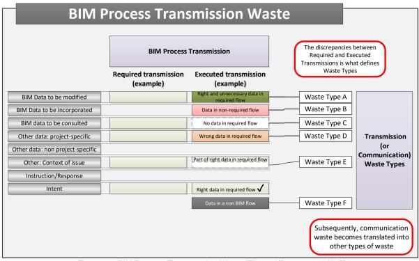
Figure 46 BIM Process Transmission Waste: The 6 different types (A-E)
