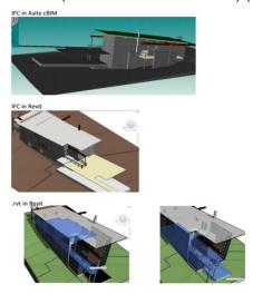
Figure 22 Visual inspection: comparing original .rvt model with IFC exports in Revit and Asite cBIM
