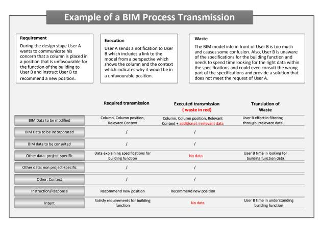
Figure 38 An example of a BIM process transmission with Transmission Waste
