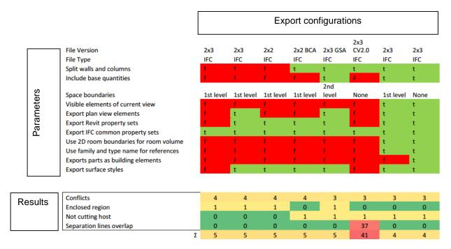
Figure 24 Warnings from different IFC export settings (f=parameter/option disabled, t=parameter/option enabled)
