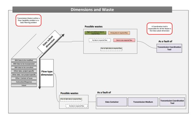
Figure 5040 Dimensions and Waste: The two dimensions of Waste are the Flow Type Dimension and the Data Subset Dimension
