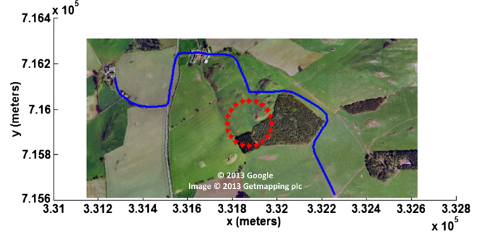
Fig. 3. The trajectories of the simulated UAV (red stars) and vehicle (blue line) movements. The satellite image is taken from Google Earth and geo-referenced. (For interpretation of the references to colour in this figure legend, the reader is referred to the web version of this article.)
