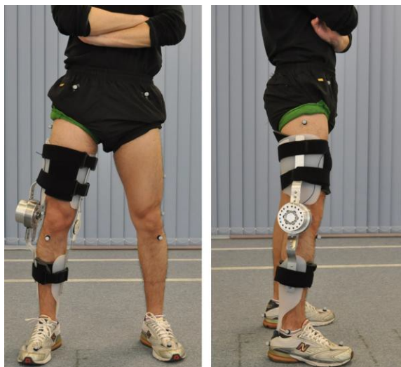
Fig. 3 Integration of knee brace to the user and placement of reflective markers.
