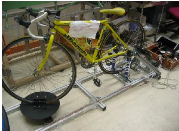
Fig. 1. The setup of the virtual cycling simulator.
