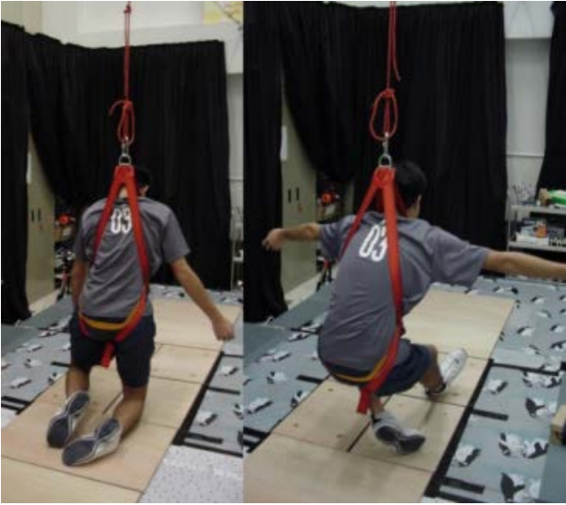
Figure 3 – Subject trying the harness to make sure it can arrest him in case of a fall
